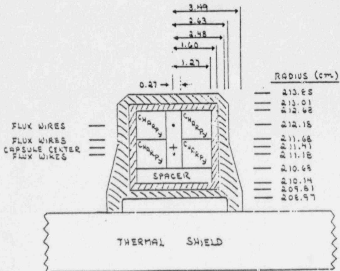
Figure III-5. Surveillance capsule geometry
