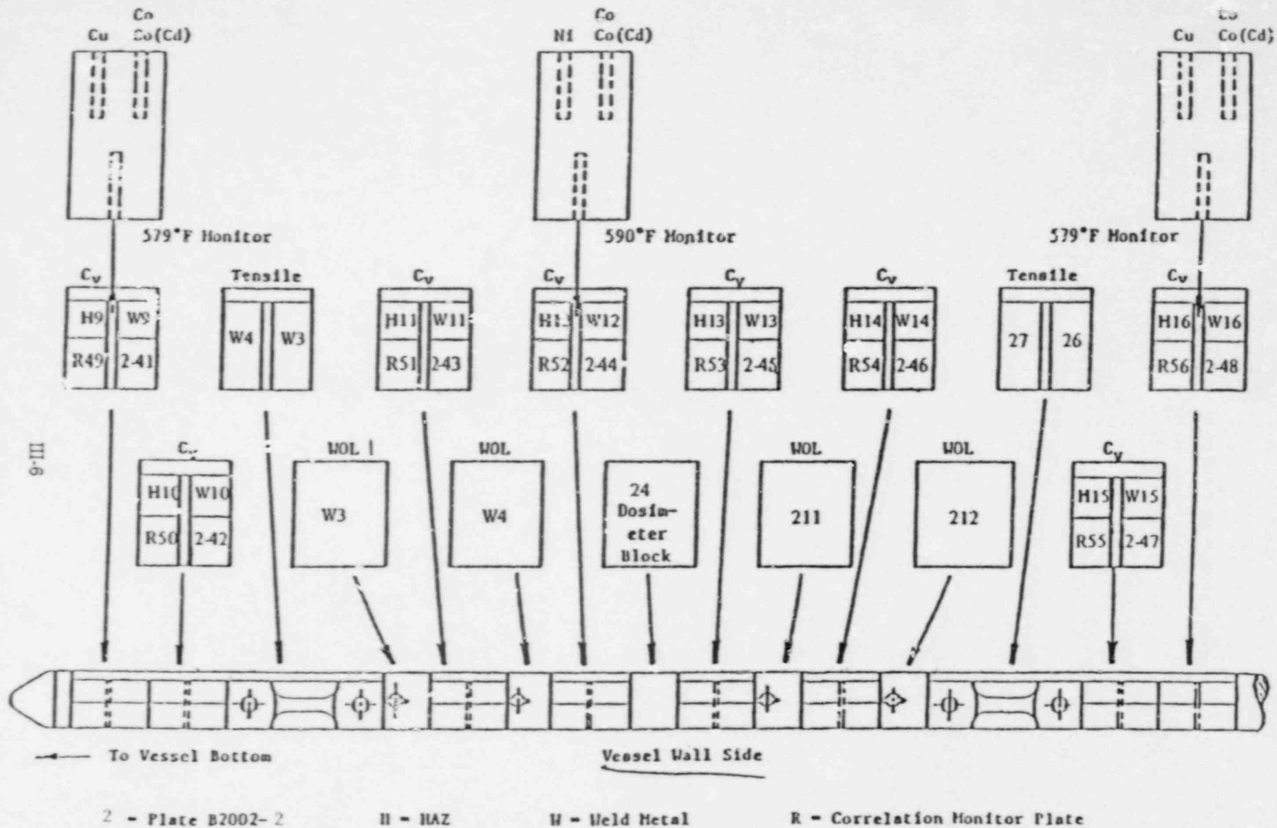
Figure III-4. Arrangement of specimens in Capsule V
