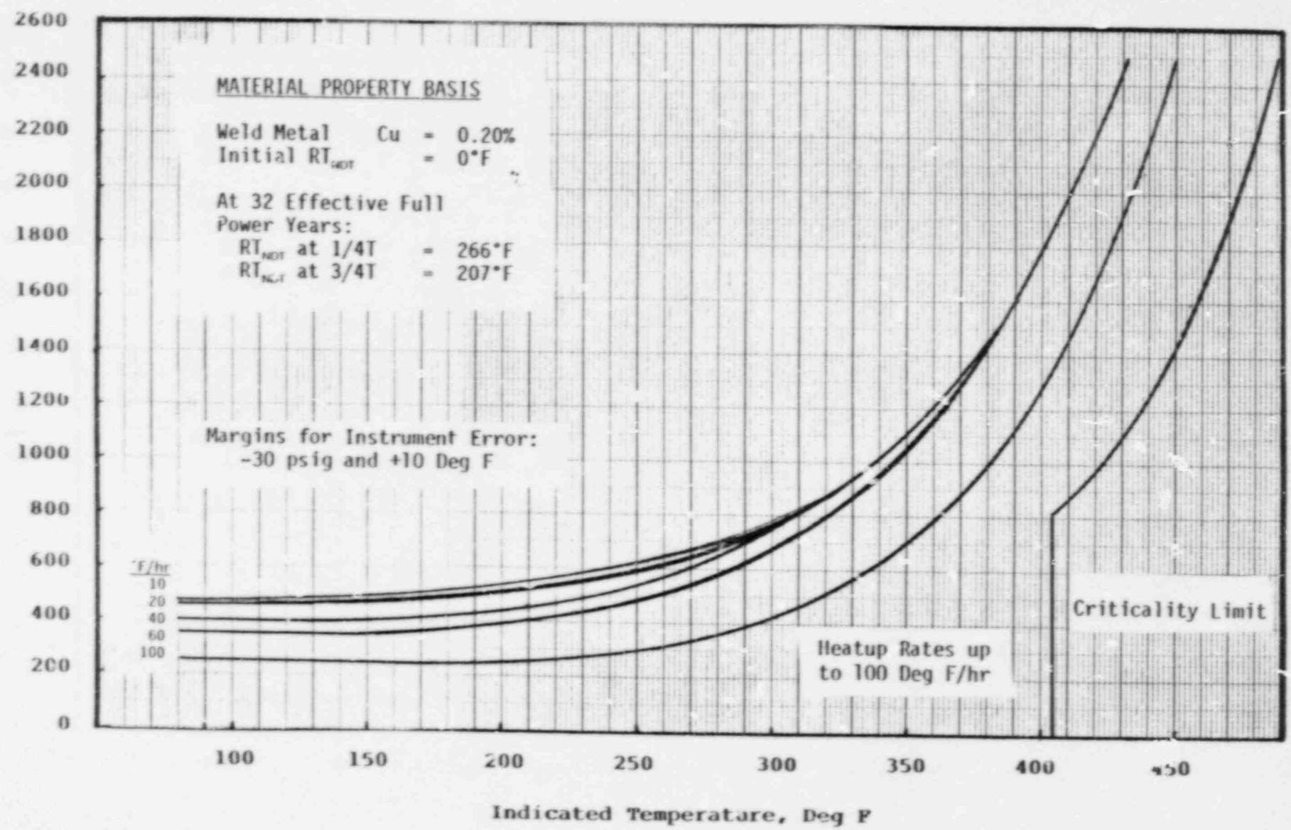
Figure VI-1. Indian Point Unit No. 2 Reactor Coolant Heatup Limitations Applicable for Periods Up to 32 Effective Full Power Years (With Criticality Limit)
