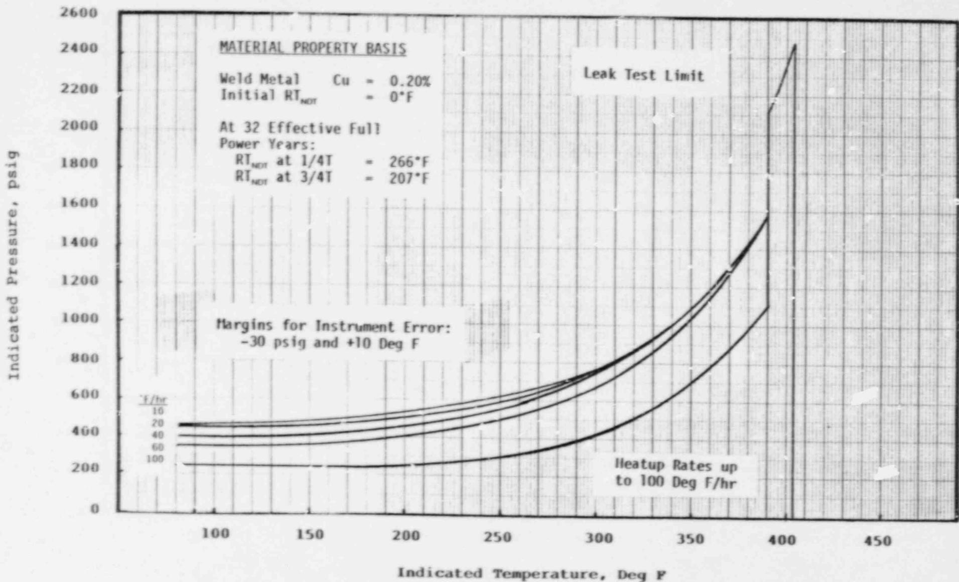
Figure VI-3. Indian Point Unit No. 2 Reactor Coolant Heatup Limitations Applicable for Periods Up to 32 Effective Full Power Years (With Leak Test Limit)
