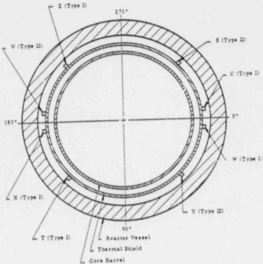
Figure III-1. Arrangement of surveillance capsules in the pressure vessel
