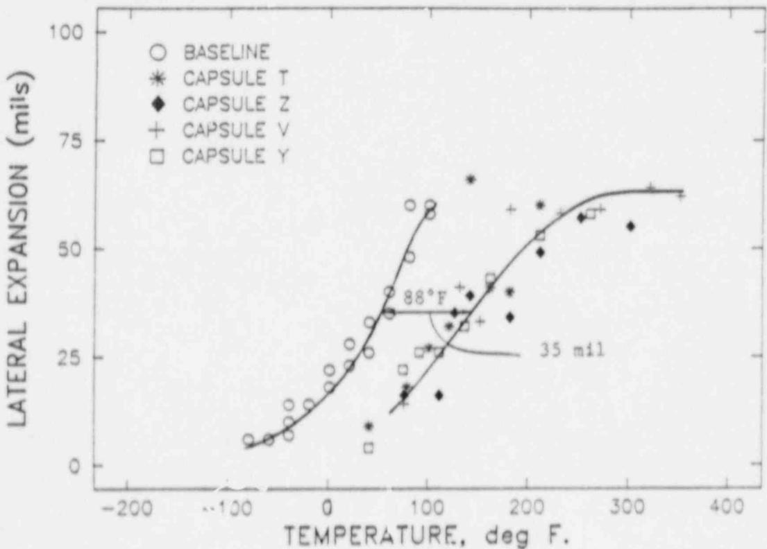
Figure IV-5. Radiation Response of Indian Point No. 2 Correlation Monitor Material
