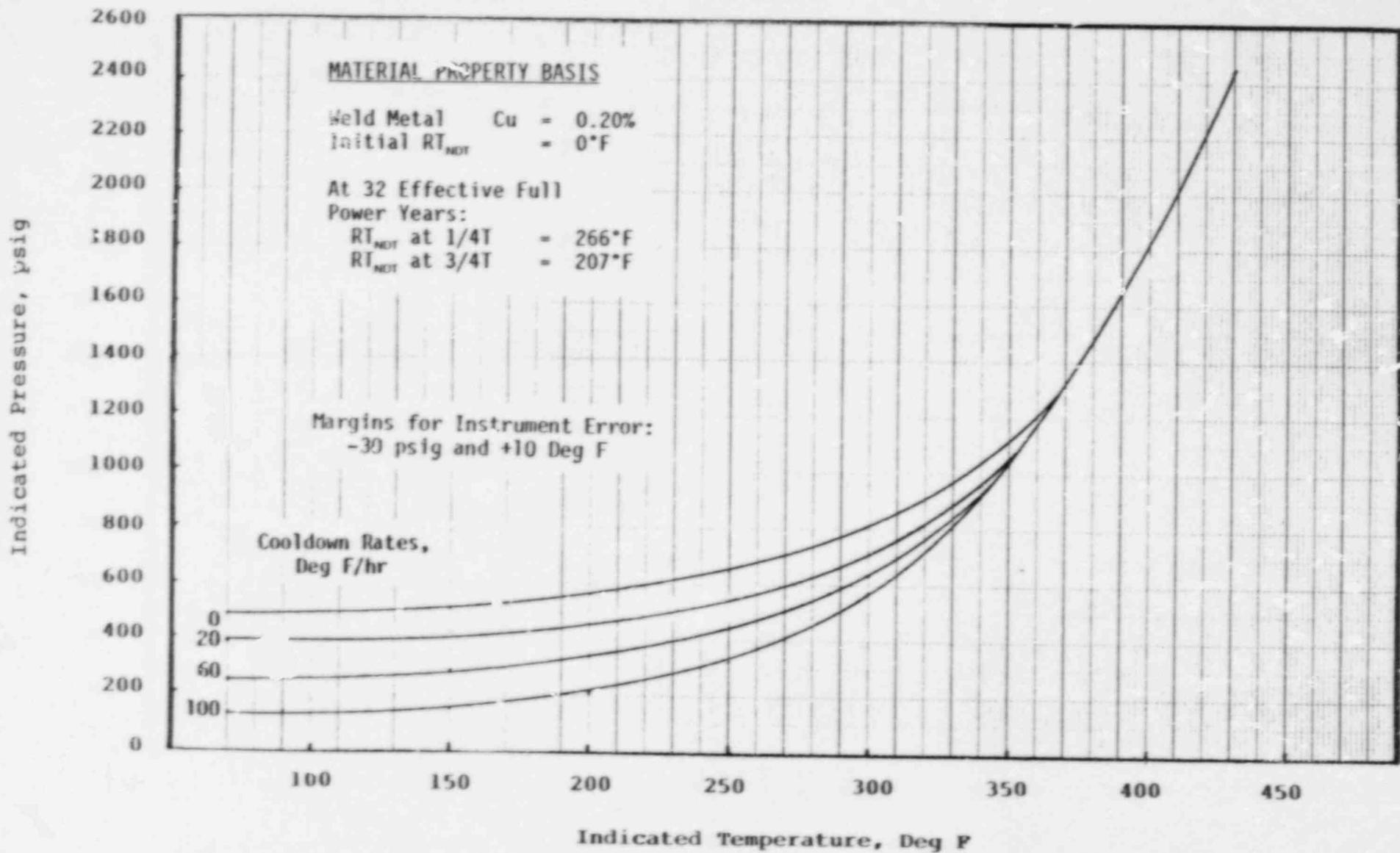
Figure VI-2. Indian Point Unit No. 2 Coolant Cooldown Limitations Applicable for Periods Up to 32 Effective Full Power Years
