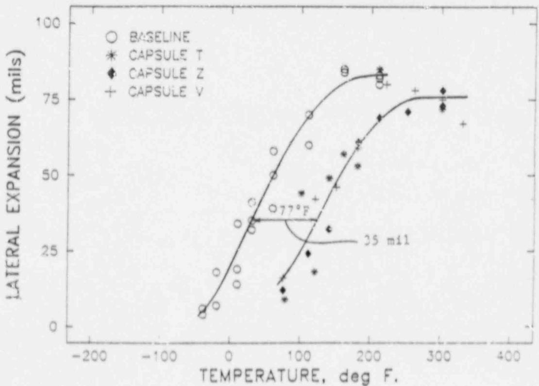
Figure IV-2. Radiation Response of Indian Point Unit 2 Shell Plate B2002-2
