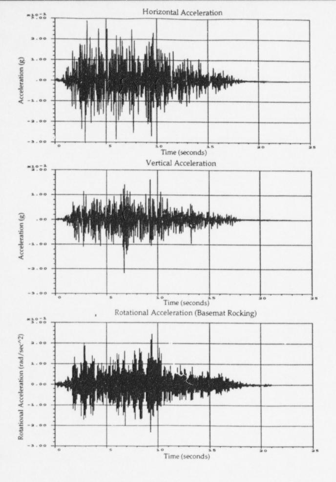
Figure 8. Post-Test Input Acceleration Records for S1(H+V)+LOCA 93
