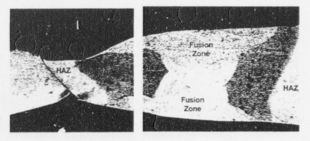
Figure 13. Cross-section through large tear @ equipment hatch
