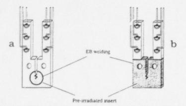
Fig.2 Miniaturised CTs with inserts of irradiated material with (a) disc and (b) square geometry
