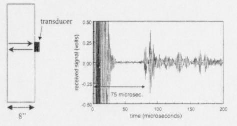
Figure 8 - Simulated UT test, setup and measured return.
