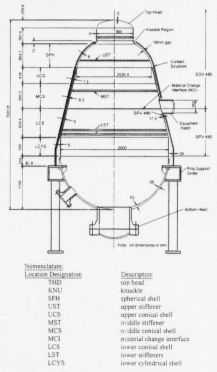
Figure 1. Elevation view of the SCV/CS assembly
