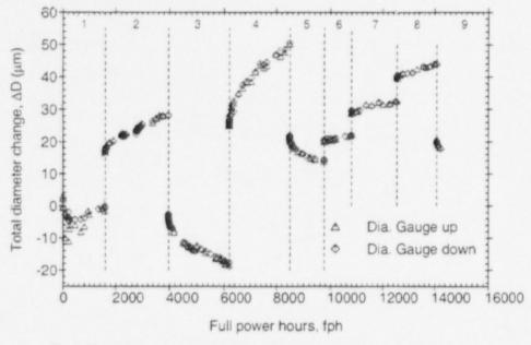
Fig. 6 Creep response of cladding tube subjected to compressive and tensile stress. The recurrence of primary creep can be noted.
