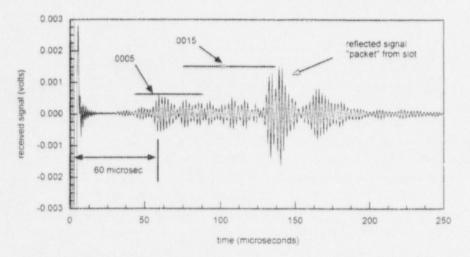
Figure 25 - Reflected signal from an embedded rectangular slot.
