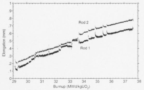
Fig. 5 Cladding elongation at steady state power of 35 kW/m for a PWR fuel rod with medium burnup
