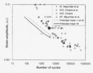
Figure 3 : Random fatigue damage growth in A106 Gr B steel at 288C in air
