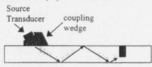
Figure 3 - Procedure used in Angle Beam Inspections.
