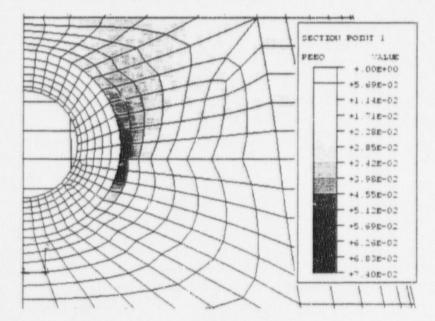
Figure 19. Equivalent plastic strain contours around the equipment hatch from the posttest analysis
