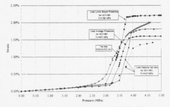
Figure 12. Hoop strains @ upper conical shell section (UCS), El. 2536 mm
