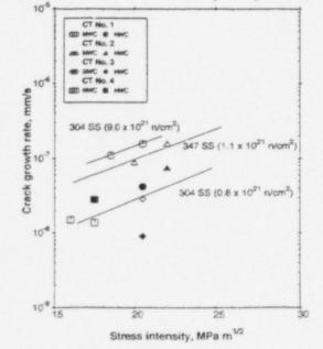
Fig. 3 Crack growth rates measured in irradiated CTs at different stress intensities and in NWC and HWC.
