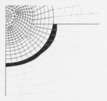
Figure 18. Local 3D equipment hatch model with SPV490 HAZ elements highlighted in black
