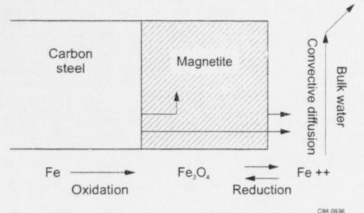
Figure 1. The flow-accelerated corrosion model (Remy and Bouchacourt 1992).
