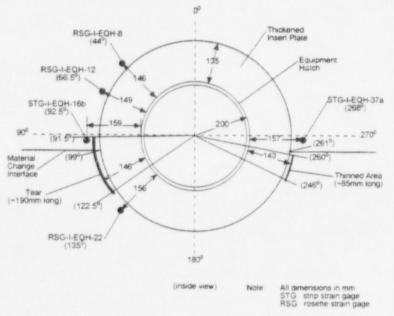
Figure 3. Interior elevation of the equipment hatch
