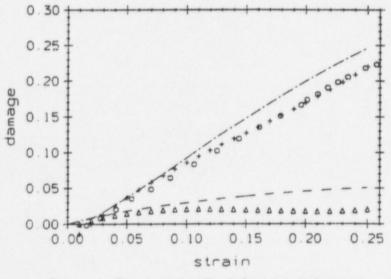
Figure 1 : Random ductile deformation damage
