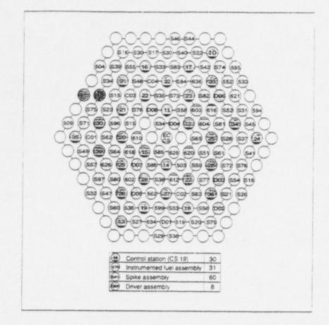
Fig. 2. Cross section of the Halden reactor core. This core configuration refers to February 1998, with totally 31 test rigs and 68 driver fuel assemblies. About half of the test rigs are operated in LWR loops.
