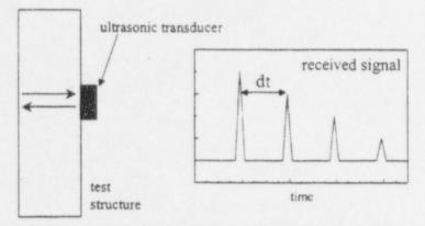
Figure 2 - Procedure used in conventional UT test.
