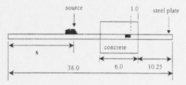
Figure 24 - Test setup for simulated field scenario.
