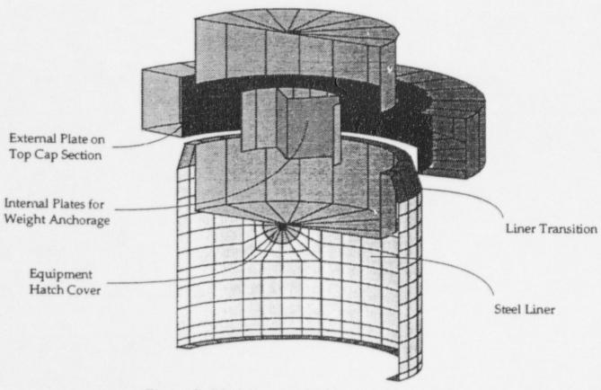
Figure 2. Modeling for the Liner and Steel Plates
