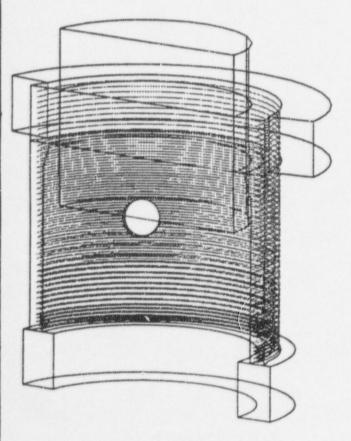
Figure 5. Modeling of Hoop Rebar
