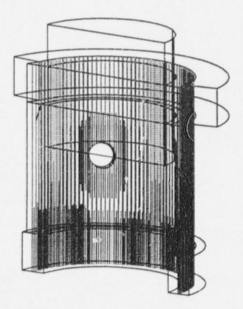
Figure 6. Modeling of Axial Rebar
