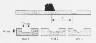
Figure 13 - Test setup for degradation shape study.
