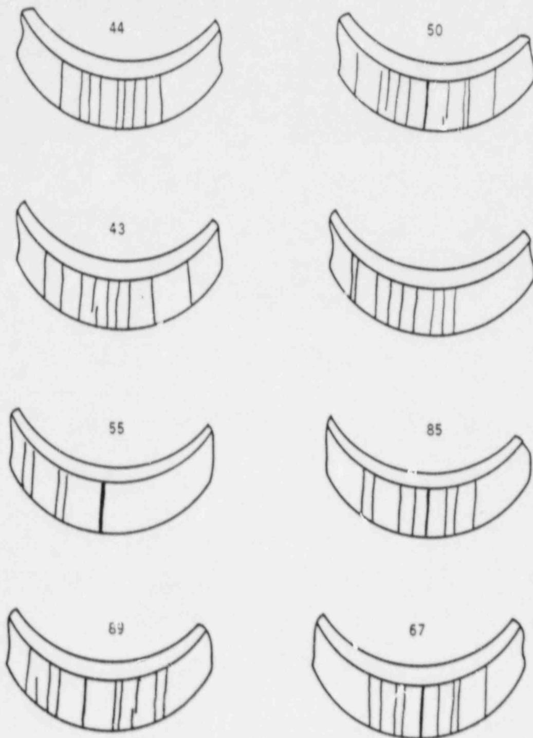
Figure 3.8 Crack patterns in as-prepared Type I Marlex CL-100 HDPE U-bend samples prior to gamma irradiation at  $4.4 \times 10^5$  rad/h. Specimen numbers given above each sketch.
