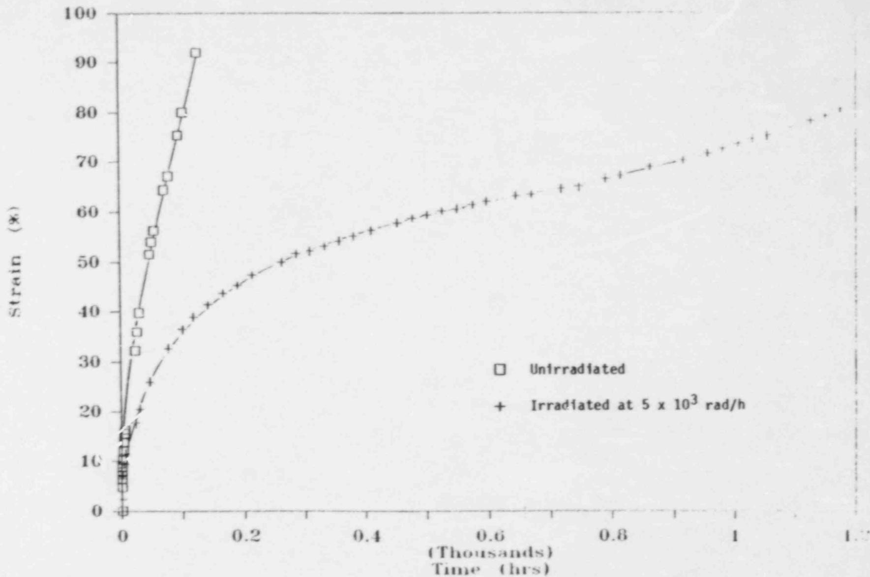
Figure 3.16 Effect of in-test gamma irradiation on the creep of Marlex CL-100 HDPE at a stress of 11.03 MPa (1600 psi).
