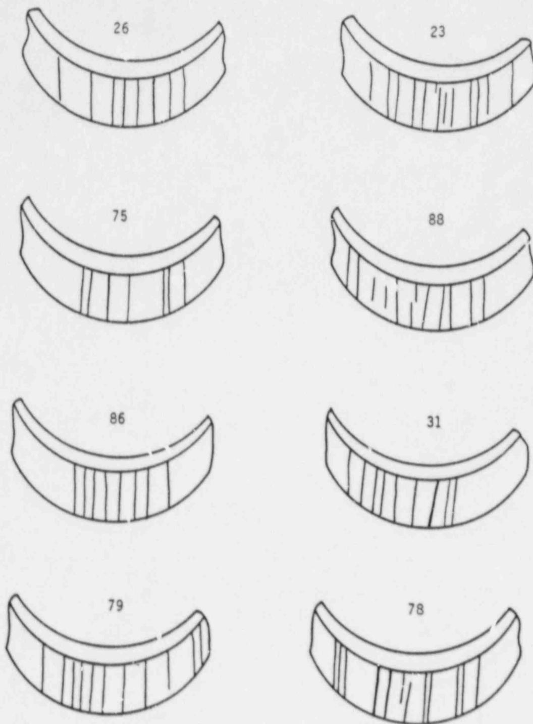
Figure 1.6 Crack patterns in as-prepared Type I Marlex CL-100 HDPE U-bend samples prior to gamma irradiation at  $8.4 \times 10^3$  rad/h. Specimen numbers given above each sketch.
