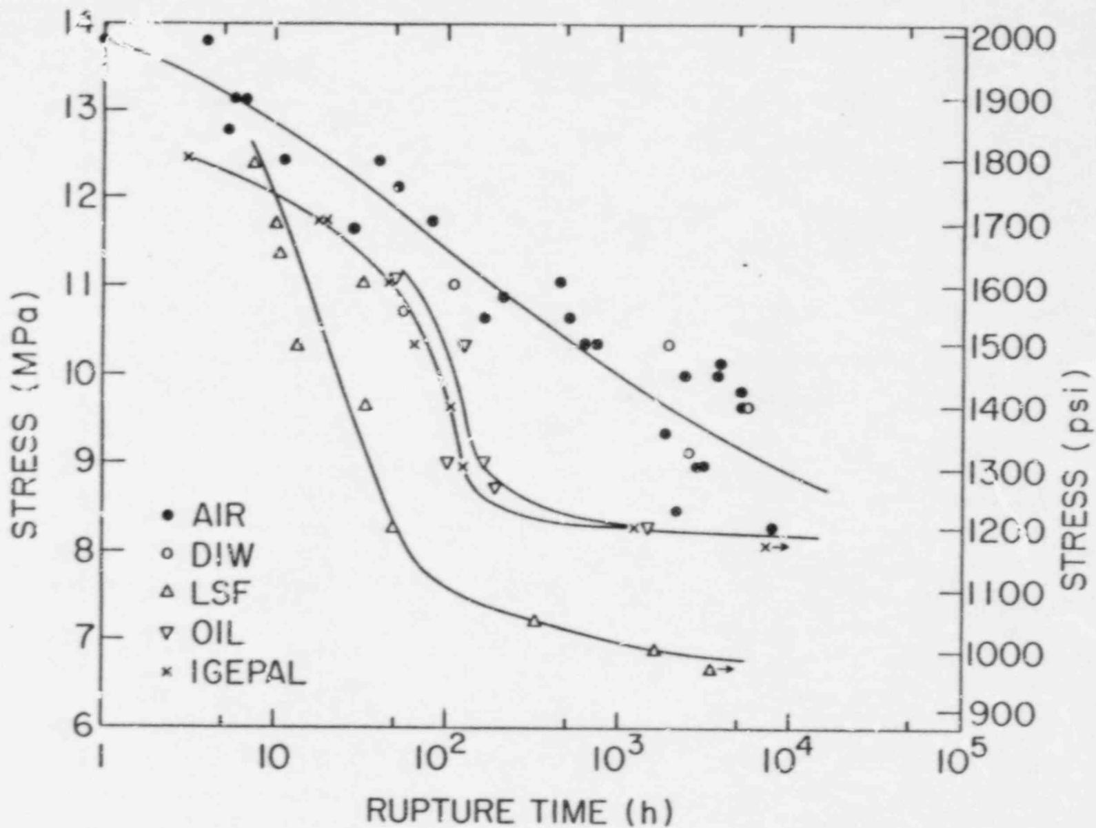
Figure 3.10 Stress-rupture results for Marlex CL-100 HDPE tested at 20 C in various environments.
