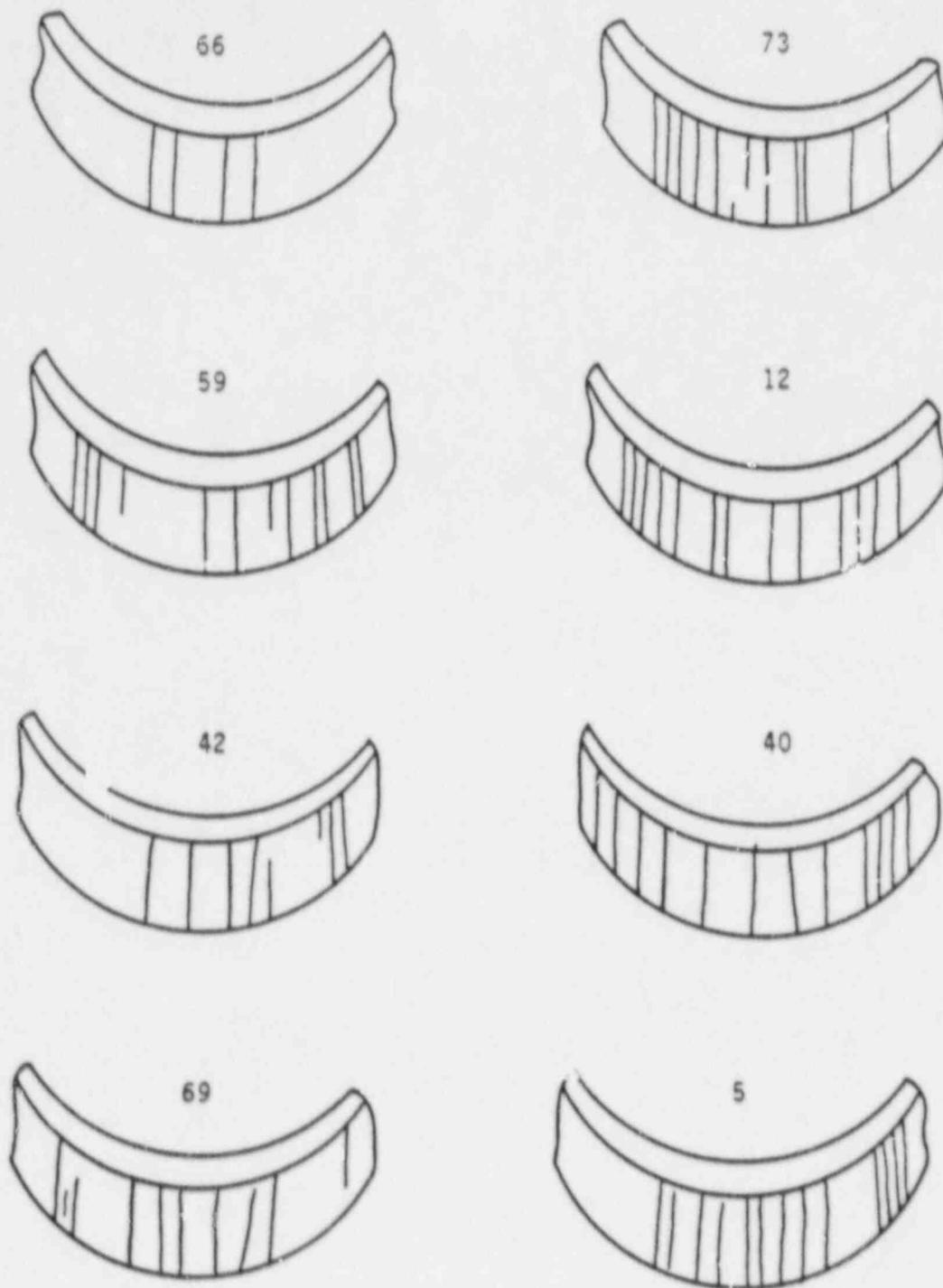
Figure 3.4 Crack patterns in as-prepared Type I Marlex CL-100 HDPE U-bend samples prior to gamma irradiation at  $1.4 \times 10^3$  rad/h. Specimen numbers given above each sketch.
