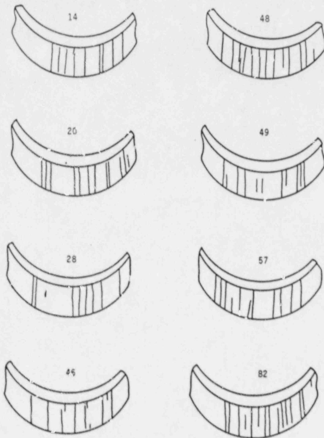
Figure 3.2 Crack patterns in as-prepared Type I Marlex CL-100 HDPE U-bend samples. Specimens are unirradiated controls. Specimen numbers given above each sketch.
