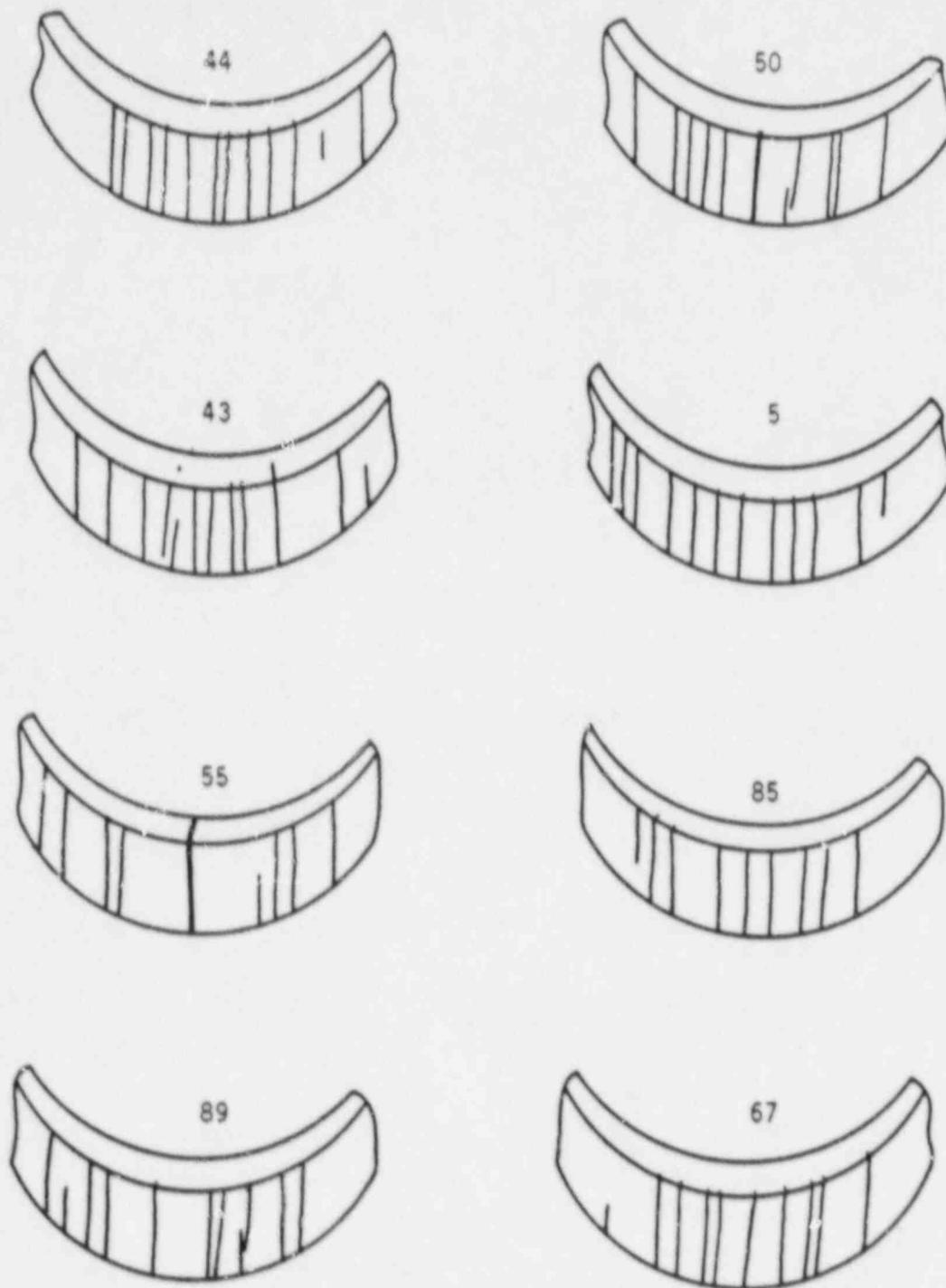
Figure 3.9 Crack patterns in Type I Marlex CL-100 HDPE U-bend samples after irradiation to  $3.1 \times 10^9$  rad at a dose rate of  $4.4 \times 10^5$  rad/h. Specimen numbers given above each sketch.
