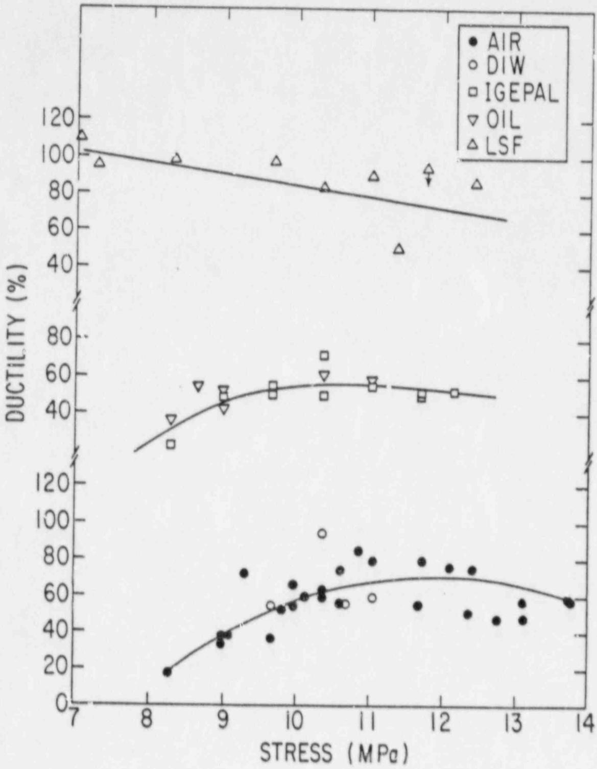
Figure 3.11 Elongations at failure for Marlex CL-100 HDPE tested at 20 C in various environments.
