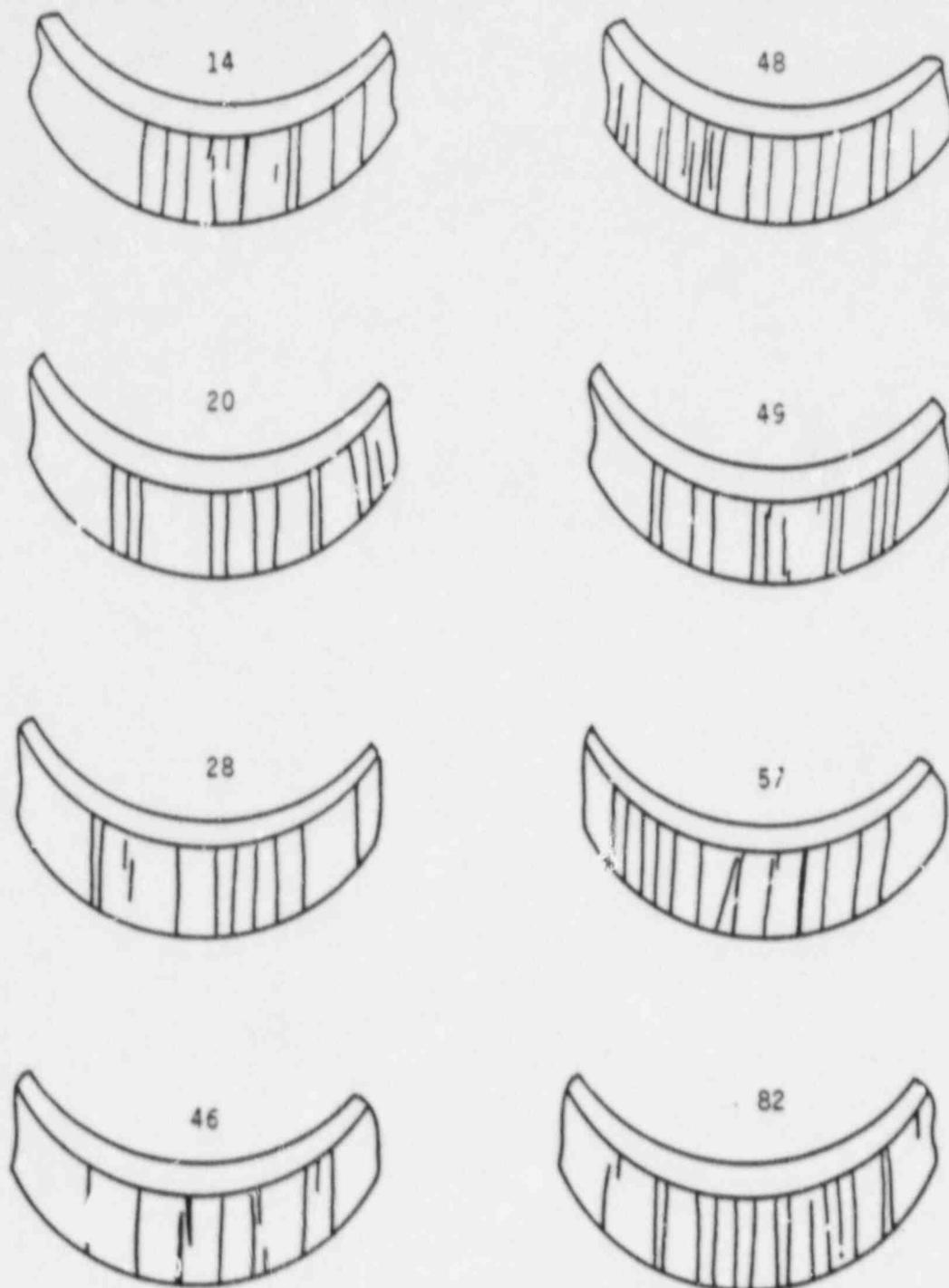
Figure 3.3 Crack patterns in unirradiated Type I Marlex CL-100 HDPE U-bend samples held at 10 C for 530 d in air. Specimen numbers given above each sketch.
