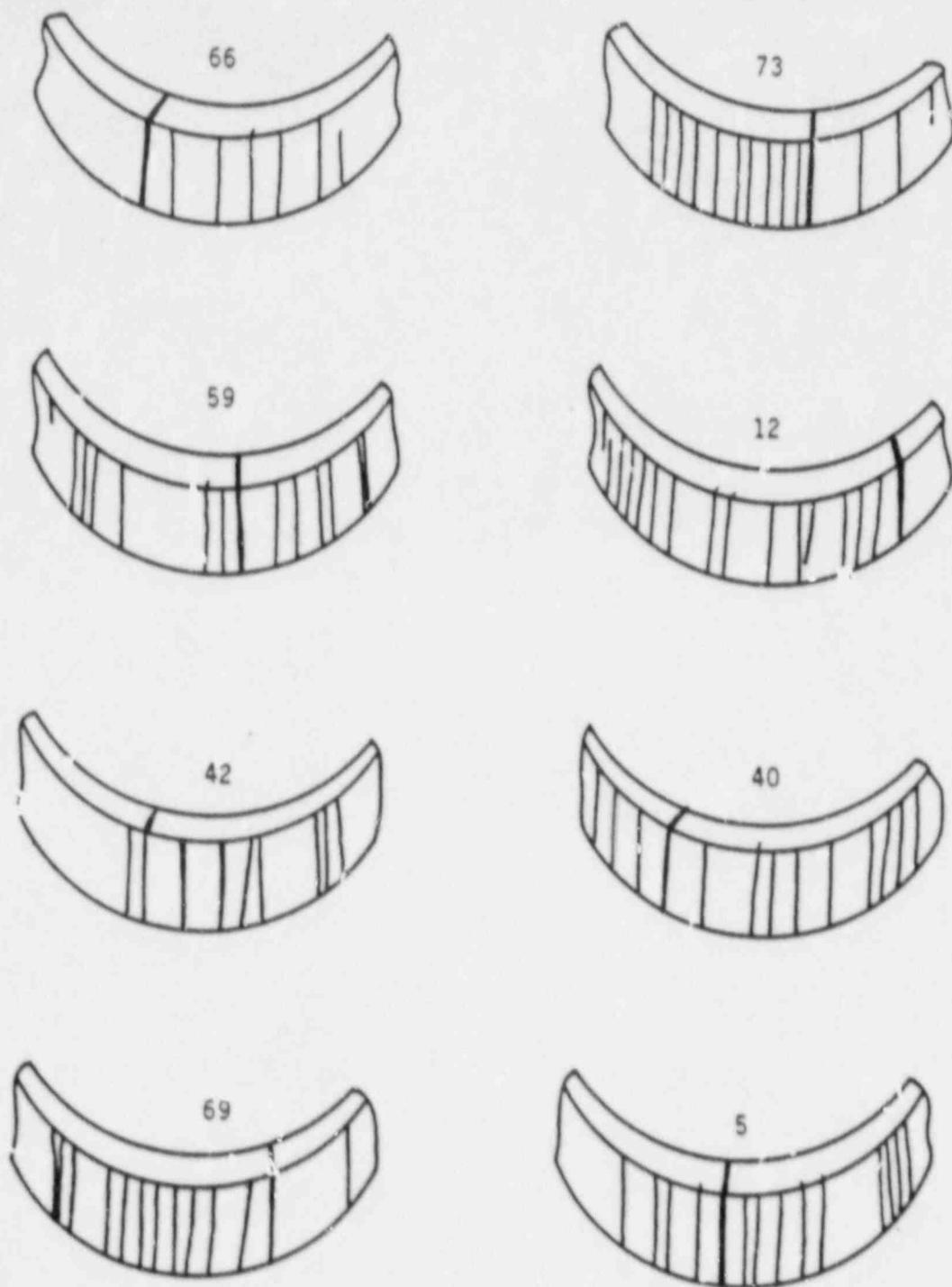
Figure 3.5 Crack patterns in Type I Marlex CL-100 HDPE U-bend samples after gamma irradiation to  $1.3 \times 10^7$  rad at a dose rate of  $1.4 \times 10^3$  rad/h. Specimen numbers given above each sketch.
