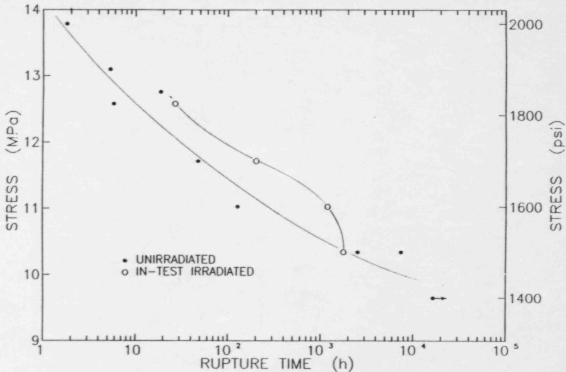
Figure 3.14 Effect of in-test gamma irradiation at  $5 \times 10^3$  rad/h on the stress-rupture behavior of Marlex CL-100 HDPE.
