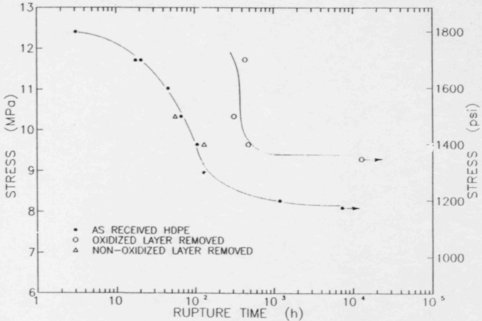
Figure 3.12 Effect of removing the oxidized and the non-oxidized surface layers on the stress rupture of Marlex CL-100 HDPE in Igepal CO-630.
