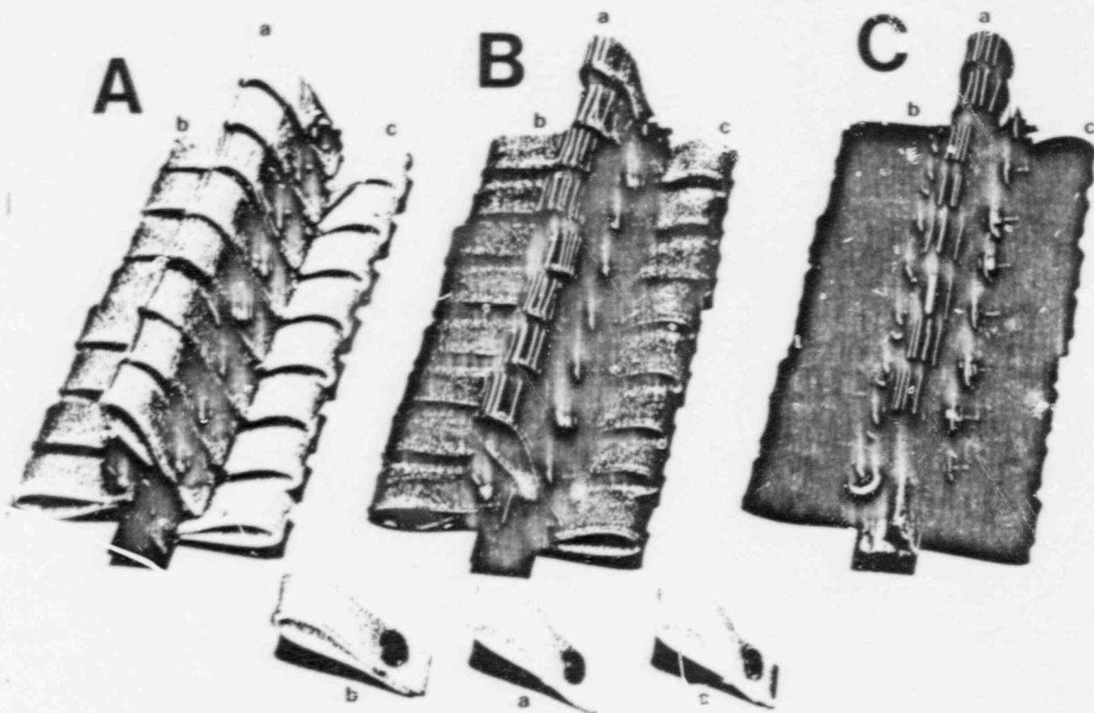
Figure 3.1 Appearance of Type I (a), Type II (b), and Type III (c) Marlex CL-100 HDPE U-bend specimens gamma irradiated to  $2.1 \times 10^6$  rad (A),  $1.3 \times 10^7$  rad (B), and  $6.7 \times 10^8$  rad (C). Individual unirradiated Type I, Type II, and Type III control specimens are shown at the bottom of the figure. Magnification 0.8 X.
