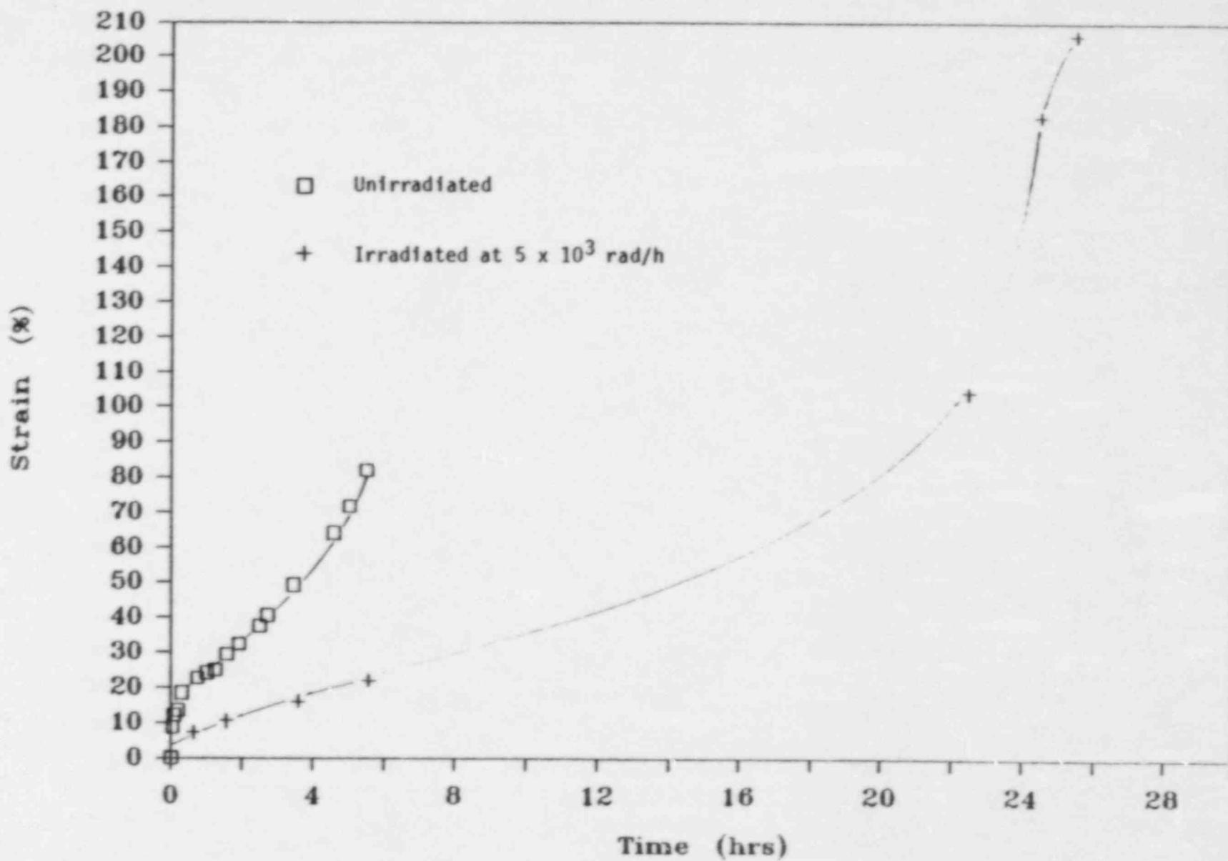
Figure 3.18 Effect of in-test gamma irradiation on the creep of Marlex CL-100 HDPE at a stress of 12.58 MPa (1825 psi).
