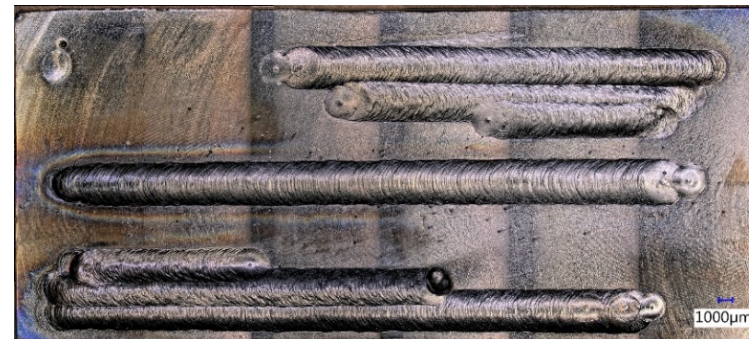
Welds performed at WEC on irradiated sample with ~3 appm He
