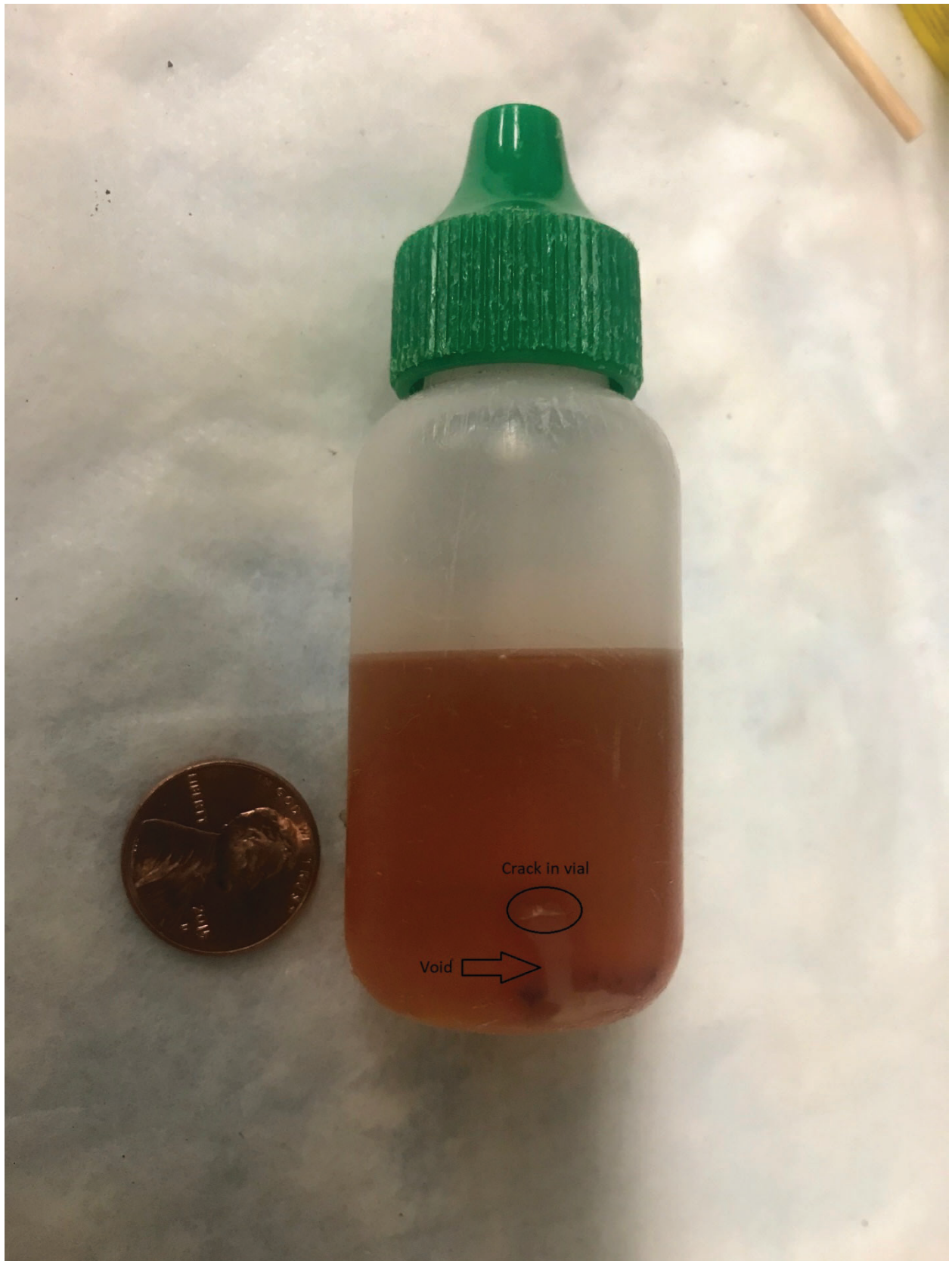
Leaking Cs-137 dose calibrator source with a 5 mm crack and void area
