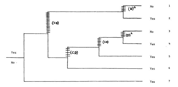
NSIC 150271 - Sequence of Interest of Both RHR Service Water Pumps Inoperable at Brunswick 2  $^1$ For success the operator must rack the pumps backin within 2-24 hours.
