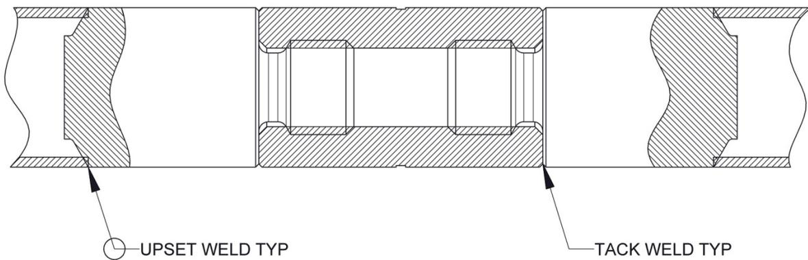
Figure 1 – Test Rod Segment Joint Configuration
