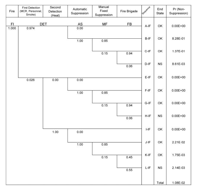
Figure 6-4 Solution for the detection-suppression event tree for NUREG/CR-6850 Example 1: interruptible fire path
