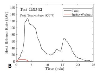
Figure 4-2 NUREG/CR-7197 experimental tests without a pre-growth period of (A) no growth and (B) no pre-growth
