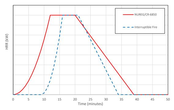
Figure 4-4 Interruptible HRR timing profile
