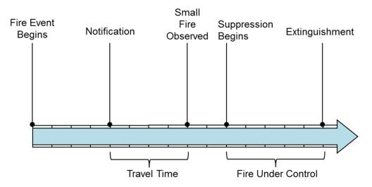
Figure 3-1 Conceptual interruptible fire timeline, not to scale
