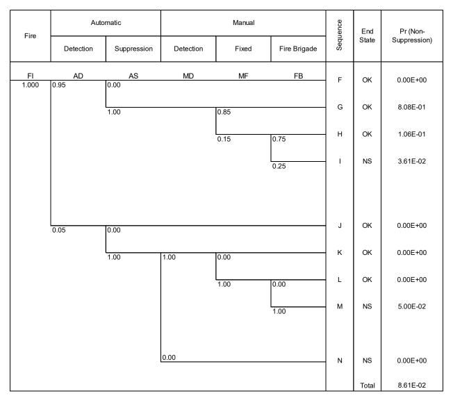
Figure 6-1 Solution for the NUREG/CR-6850 detection-suppression event tree
