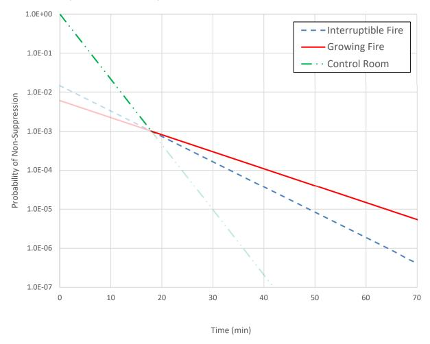
Figure 3-4 Non-suppression curve plot showing probability (logarithmic scale) versus time to suppression for MCR scenarios
