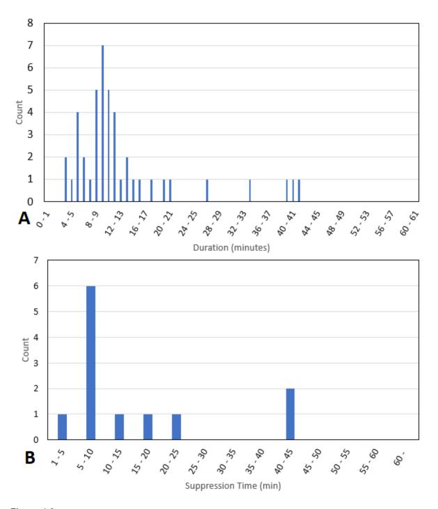
Figure 4-3 Growing fire, A) growth period duration counts, B) suppression time counts
