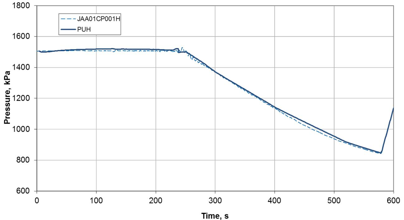
**Figure 3-3 RELAP5 Boundary Condition for Pressure in the Upper Head and SG**
