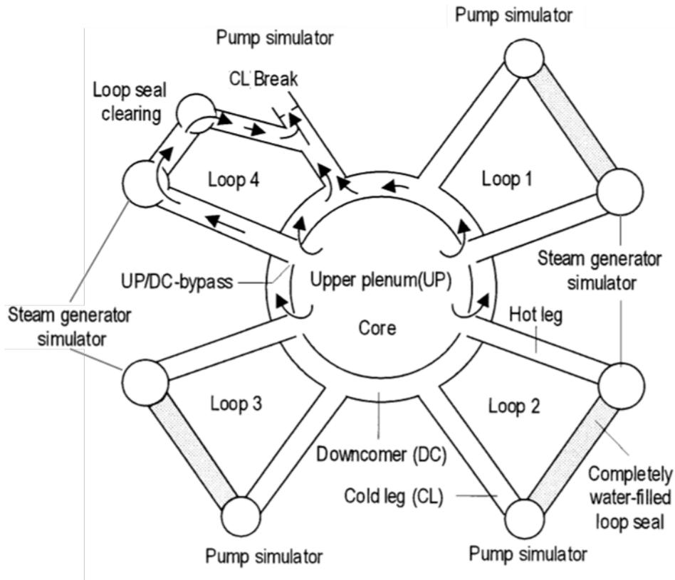
**Figure 1-2 Plan View of Steam Flow in the Primary System of a PWR During Loop-Seal Clearing with a Break in the Cold Leg of Loop 4**
