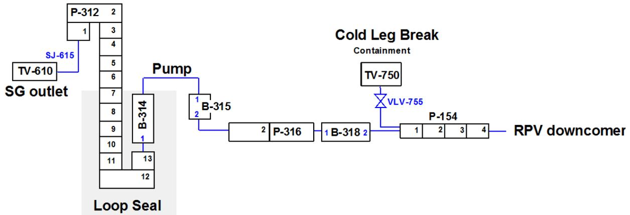
**Figure 3-2 RELAP5 Nodalization of the Loop Seal for UPTF-TRAM Test A5 ITRun2a**
