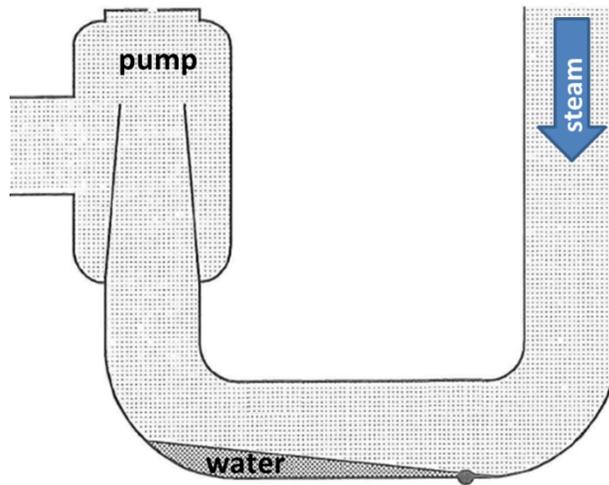
**Figure 3-6 Schematic of Water Remaining After Loop-Seal Clearing**
