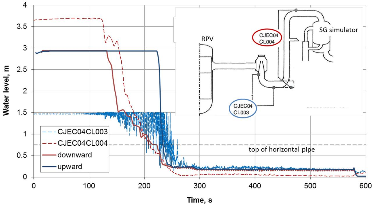
**Figure 3-5 RELAP5 Water Level in the Loop Seal**
