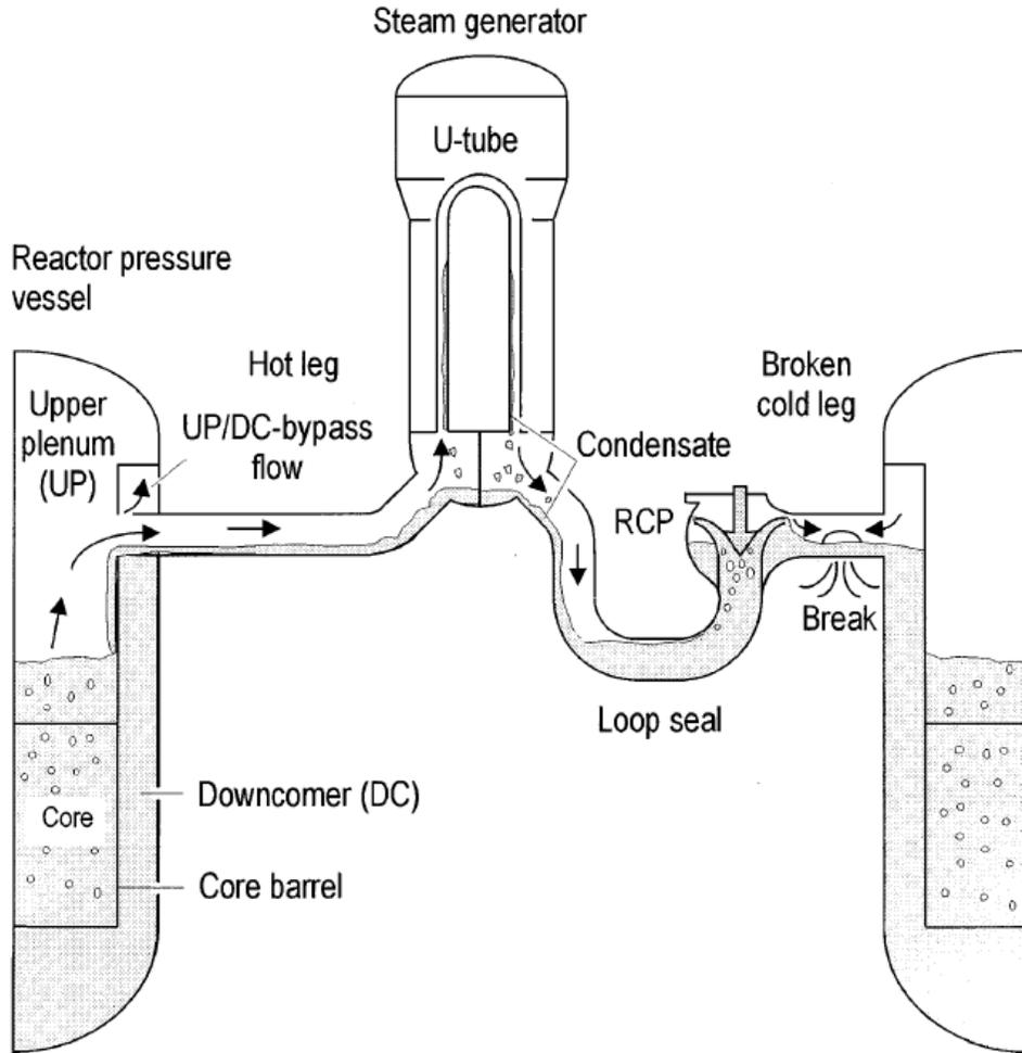
**Figure 1-1 Elevation View of Steam Flow in the Primary System of a PWR During Loop-Seal Clearing with a Break in the Cold Leg**
