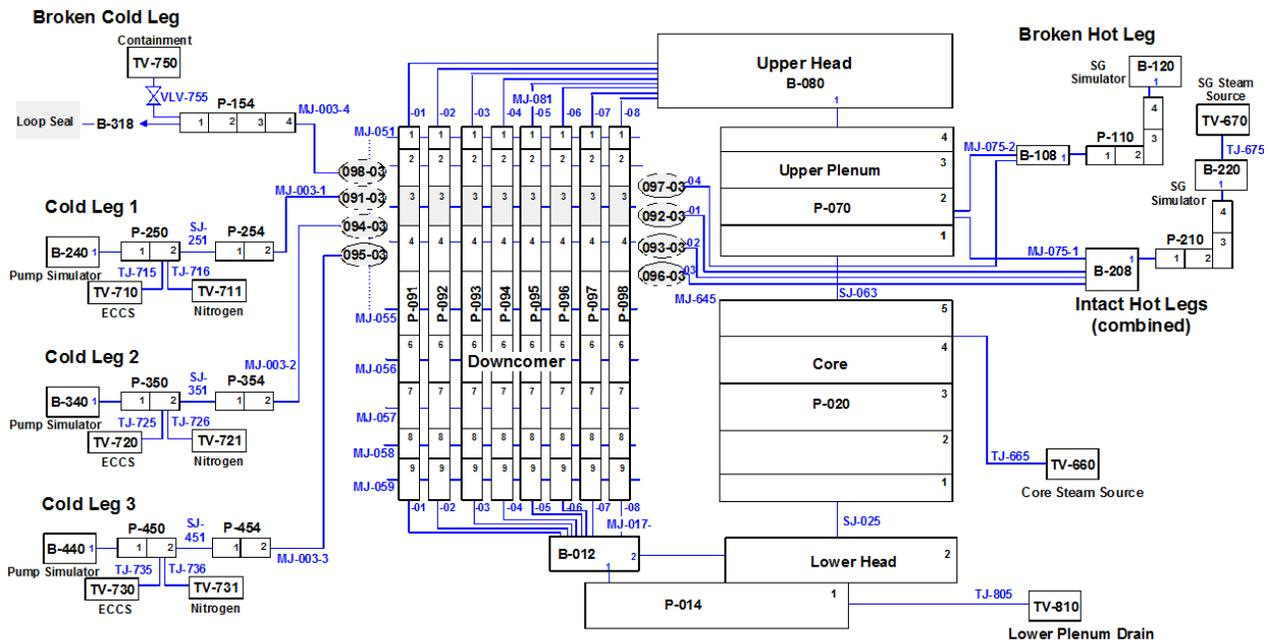
Figure 3-1 RELAP5 Nodalization of UPTF-TRAM Test A5 ITRun2a
