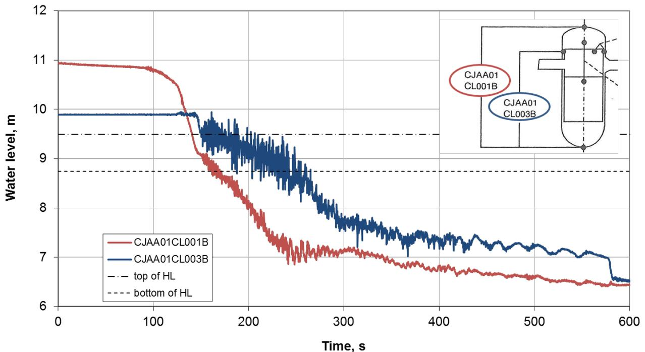
**Figure 2-3 Experimentally Derived Water Level in the Downcomer**
