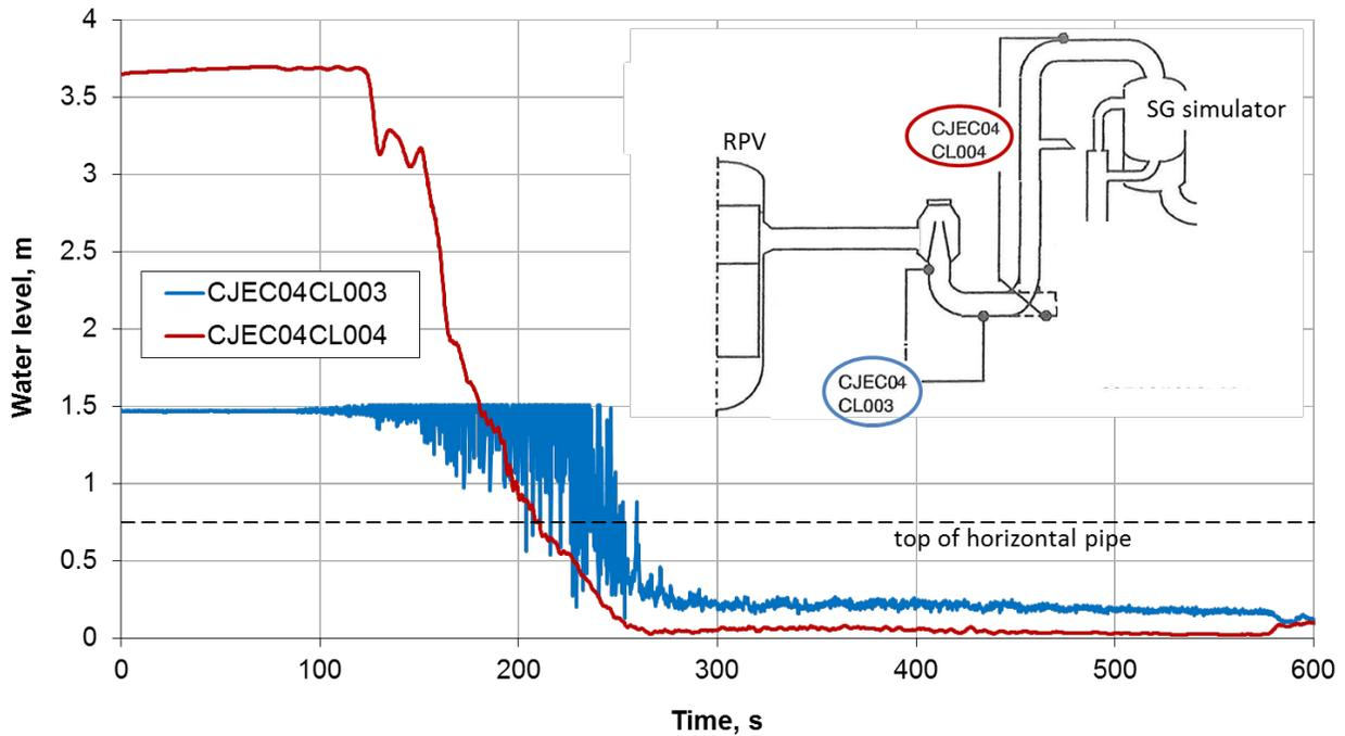
**Figure 2-4 Experimentally Derived Water Level in the Loop Seal**
