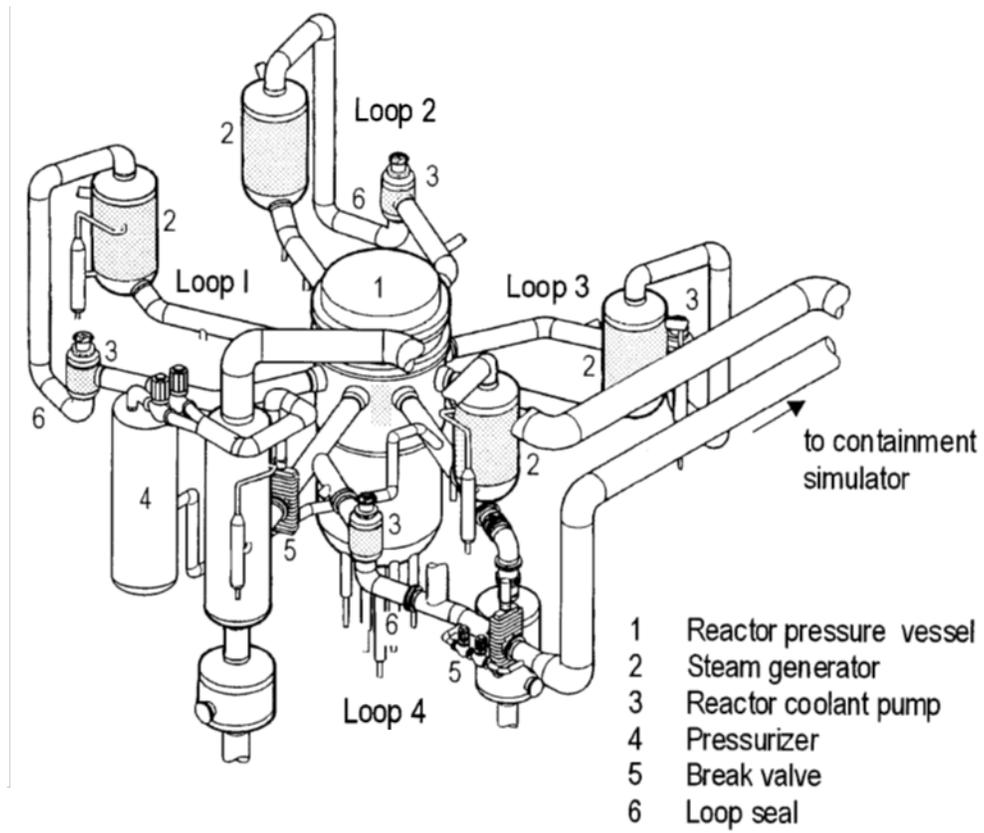
**Figure 2-1 Schematic of UPTF Indicating Primary-Side Components**
