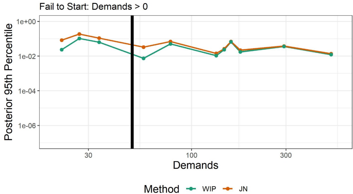
Figure C-2. 95 th percentiles for posterior WIP and JN uncertainty distributions for the probability of a component's failure to start as a function of the number of demands.
