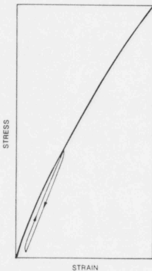
Fig. 3.12. Typical shear stress-strain curve for H440 graphite showing unload-reload behavior.
