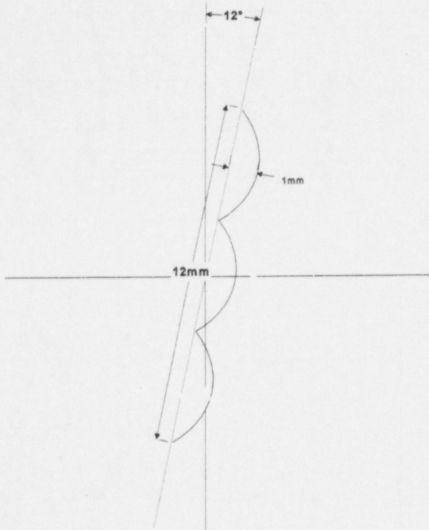
Figure C.7. 12 mm Deep Defect by 0.025 mm Width with 3 Curved Segments
