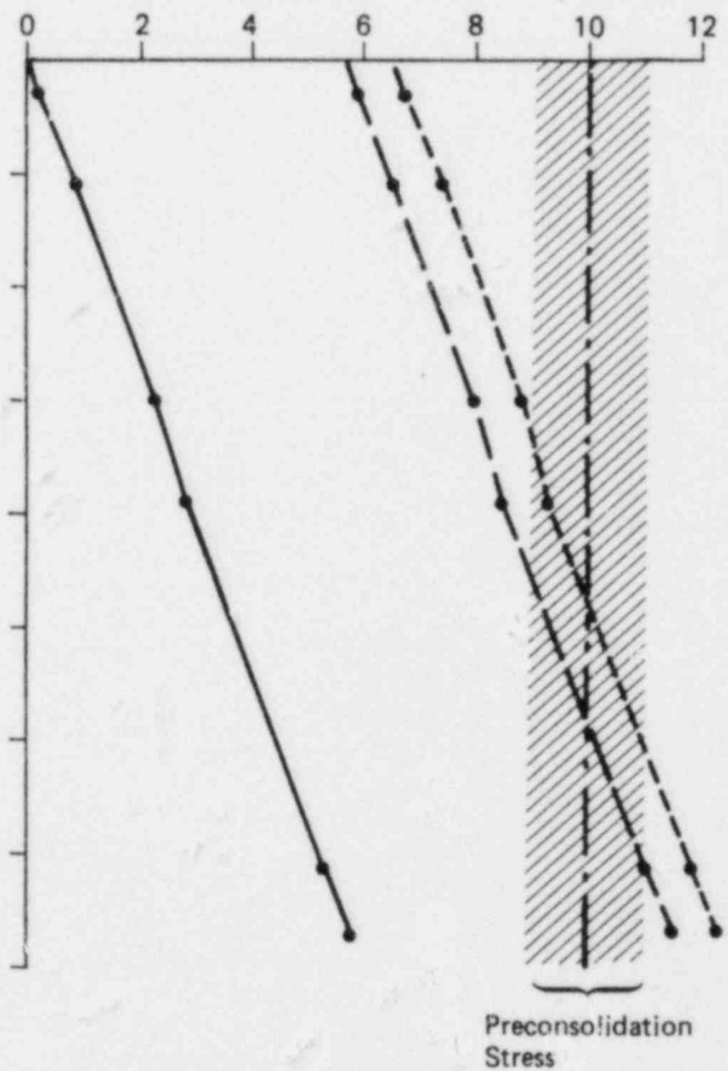
Stress Distribution at Point R (in 1000 lb/ft 2 ) (center of cell)
