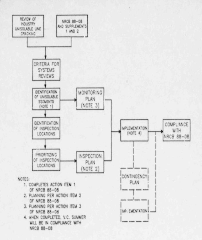
Figure 1-1. Outline of SCE&G's Plan of Action to Address NRCB 88-08 for the Virgil C. Summer Plant
