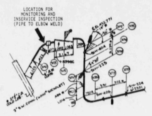
Figure 1-7. Locations for Inservice Inspection and Monitoring on the Unisolable Section of the Loop C Cold Leg Safety Injection Line
