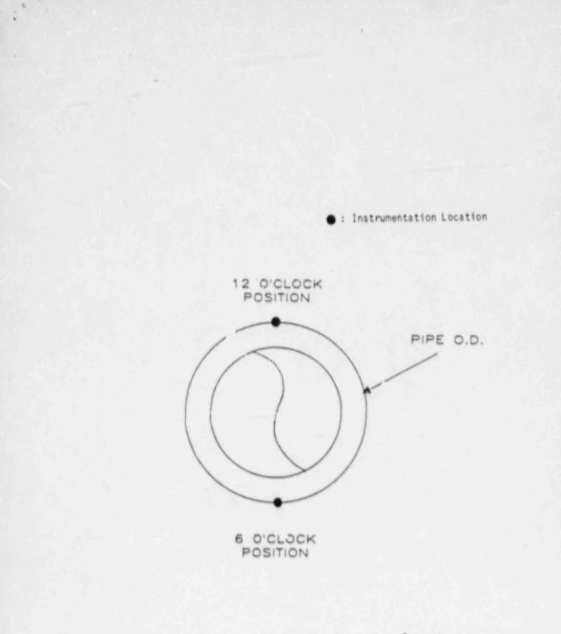
Figure 1-11. Mounting Locations for Temperature Sensors
