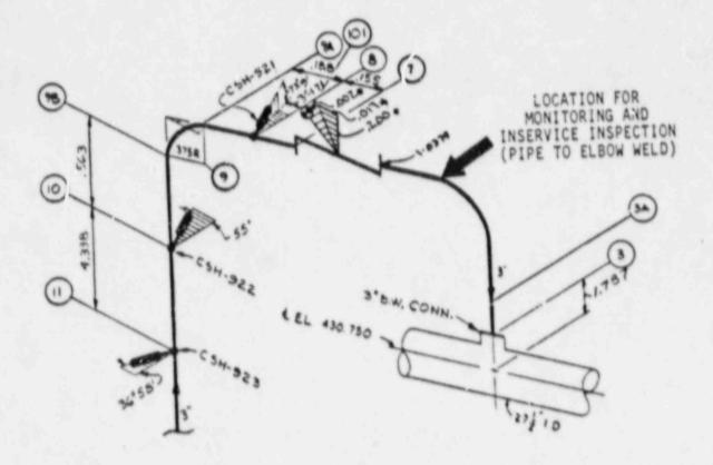
Figure 1-9. Locations for Inservice Inspection and Monitoring on the Unisolable Section of the Alternate Charging Line
