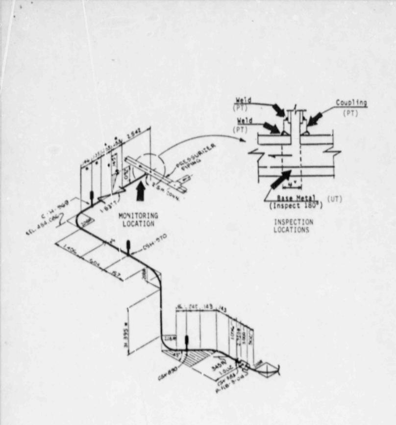
Figure 1-8. Locations for Inservice Inspection and Monitoring on the Unisolable Section of the Auxiliary Spray Line
