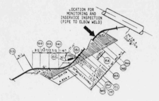
Figure 1-4. Locations for Inservice Inspection and Monitoring on the Unisolable Section of the Loop B Hot Leg Safety Injection Line
