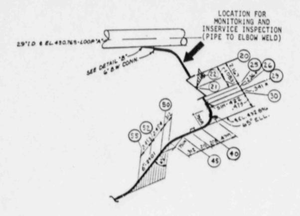
Figure 1-6. Locations for Inservice Inspection and Monitoring on the Unisolable Section of the Loop A Hot Leg Safety Injection Line
