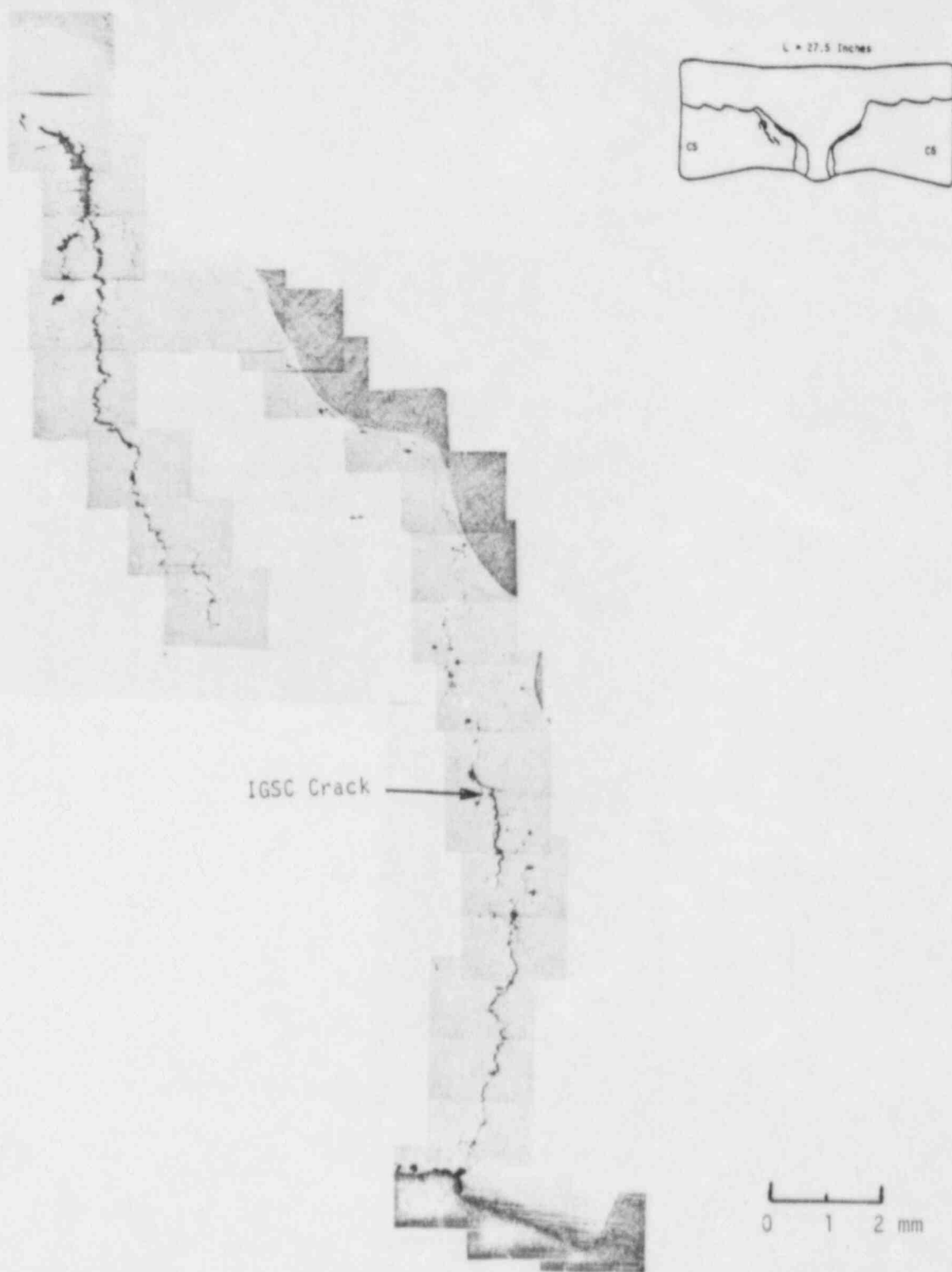
FIGURE 4.3. Cross Section of C5 Side of NC5-C6 at 27.5 Inches, Indicating a Through-Wall Depth of 86% of the Original Pipe Wall. (Crack Depth = 0.682 Inch; Total Remaining Wall = 0.396 Inch.) Source: Becker et al., EPRI NDE Center, April 1985.
