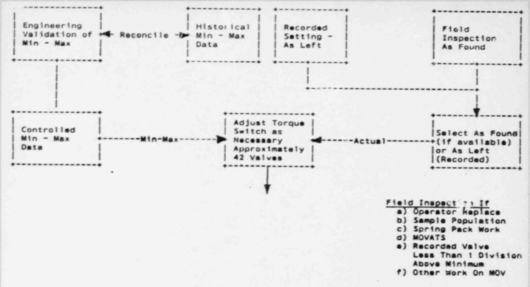
Valve Torque Switches Reset
