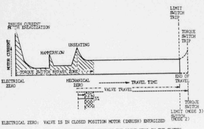
HAMMERBLOW: DOGS ON THE WORM WHEEL CONTACT THE DRIVE KEYS IN THE CLUTCH RING WITH CONSIDERABLE IMPACT.
