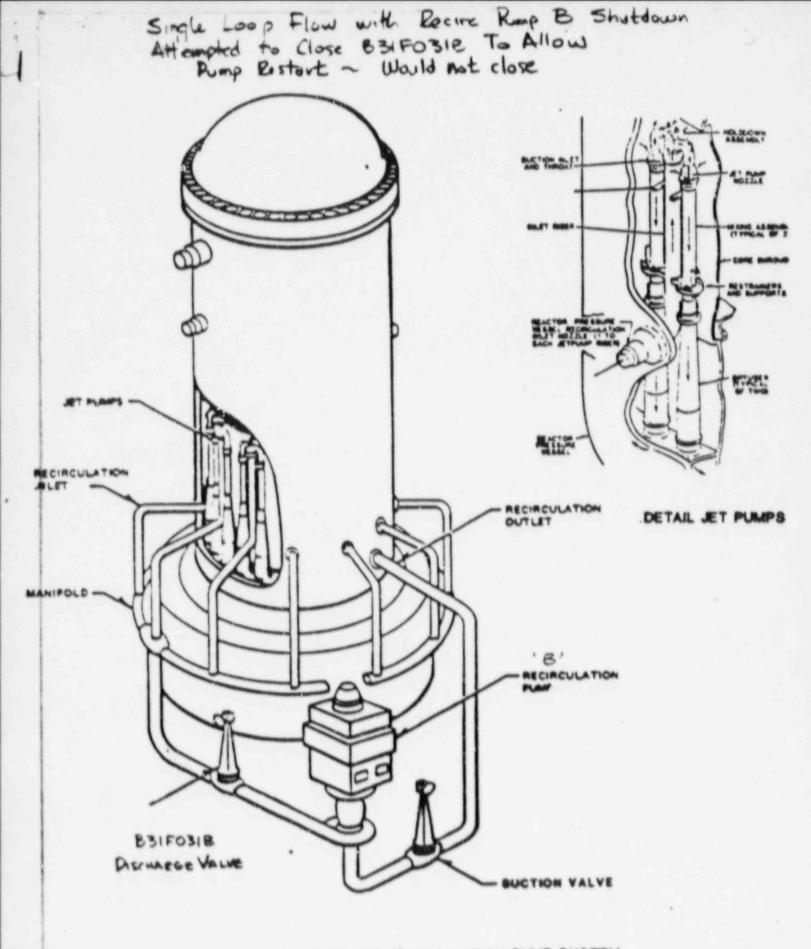
FIGURE 2-4 JET PUMPS AND RECIRCULATION PUMP SYSTEM
