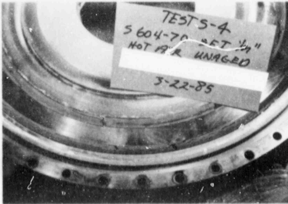
Figure A-S4.1 Test S-4 Posttest photo of plate 3 Note: Gasket degradation
