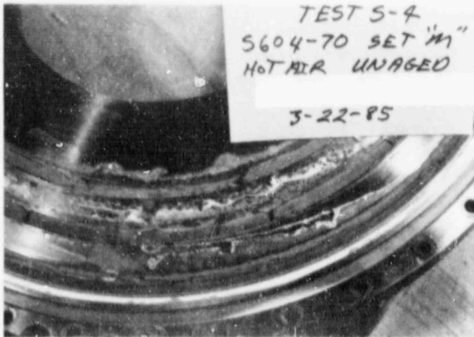
Figure A-S4.2 Test S-4 Posttest photo of plate 2 Note: Gasket degradation
