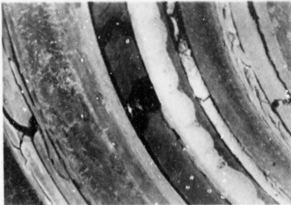
Figure A-S1.2 Test S-1 Posttest photo of plate 1 Note: Gasket degradation
