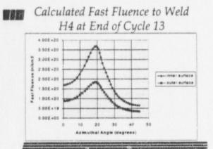
Neutron Transport Results for Shroud Welds
