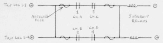
The root cause of the event was an incorrect amperage fuse (vendor: Bussman, Model Number: KLM4), which caused the trip on the MSIS 1-3 leg. The fuse was found to be a 4 amp fuse in a location where the design calls for an 8 amp fuse. An investigation is being conducted into the root cause of how and when the fuse was installed.
