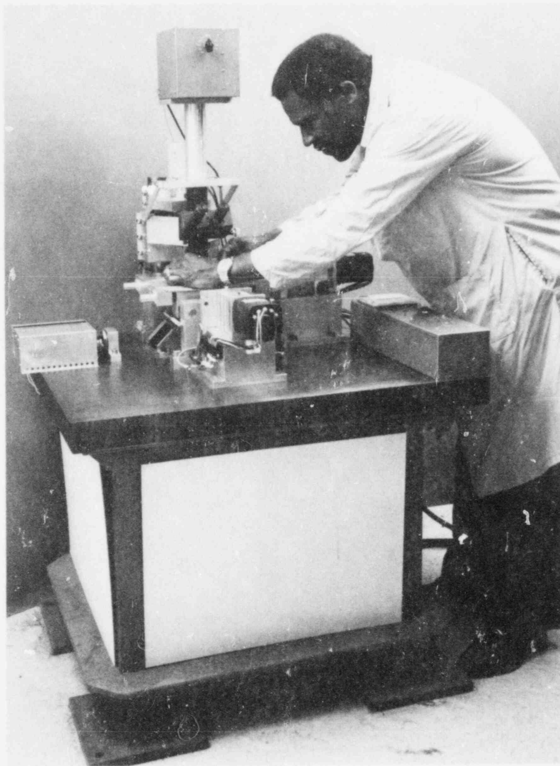
FIGURE 6. View of Hanford Optical Track Scanning (HOTS) System for SSTRs Showing Scanning Stage and Optics. Neg 8102282-4
