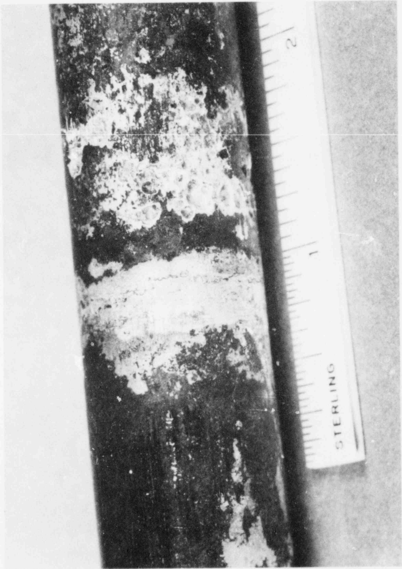
FIGURE 12. Circumferential Defects on Tube R9C60 About One Centimeter Below Deep Pits
