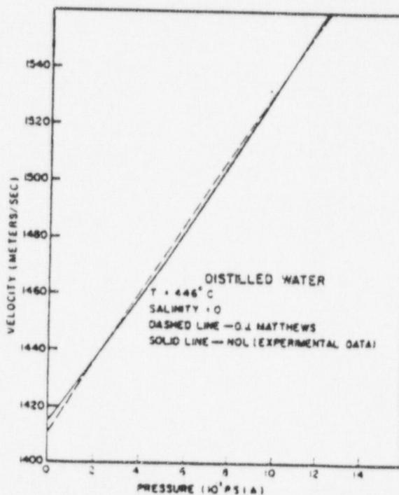
FIG. 6. Comparison of velocities predicted by D. J. Matthews and measured at NOL.
