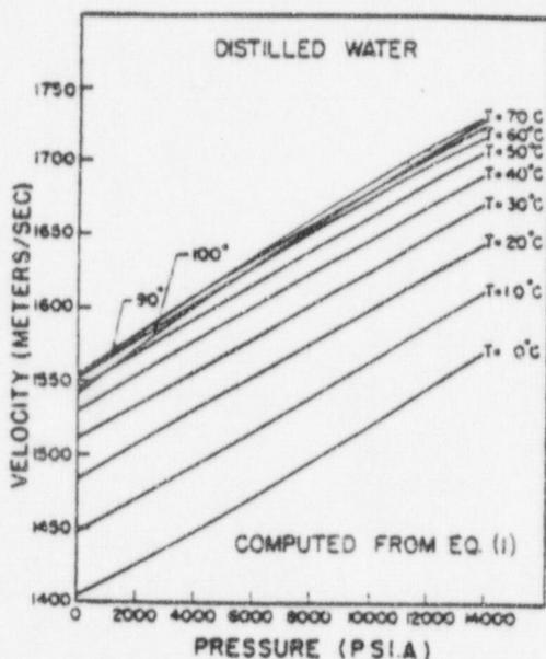
FIG. 5. Velocity of sound in distilled water as a function of pressure.
