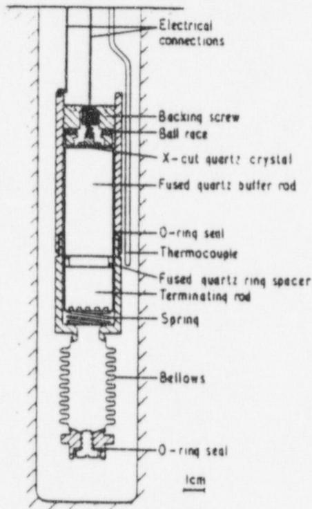
Acoustic system for measurement of velocity under high pressure.
