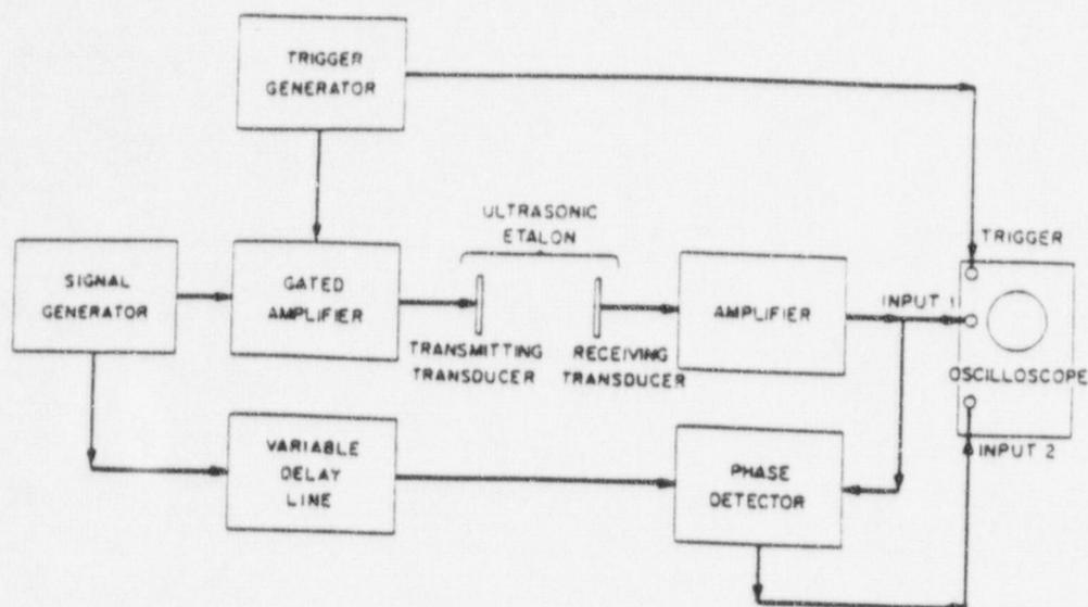
FIG. 1. Schematic diagram of ultrasonic phase-comparison circuitry.
