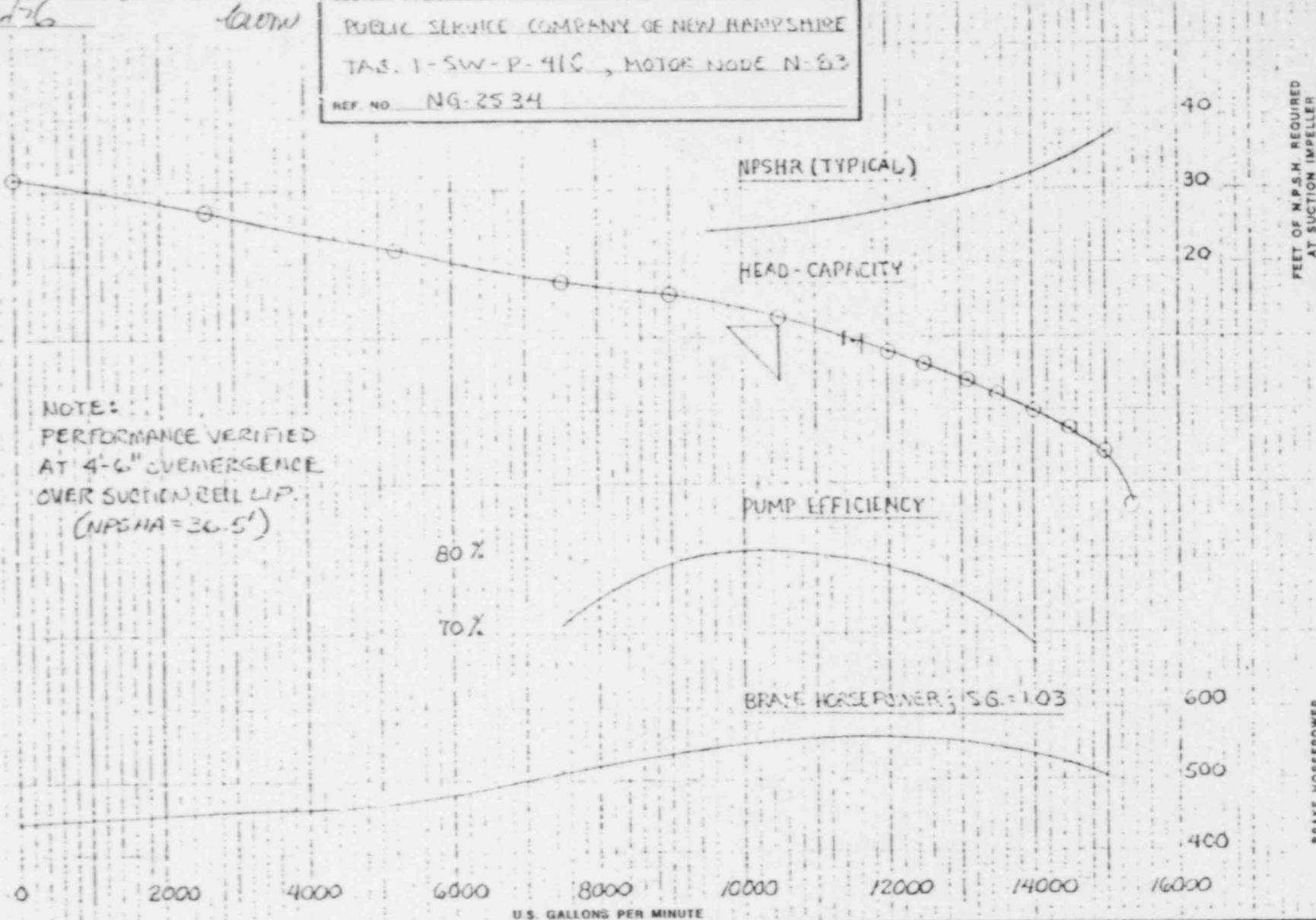
THE CAPACITY, HEAD AND EFFICIENCY
