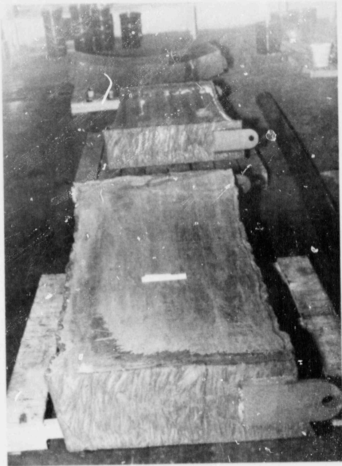
Fig. 7.21. Pilgrim Unit 2 pressure vessel pieces (arbitrarily designated as P-1, -2, and -3 with P-3 located at front of the photograph).
