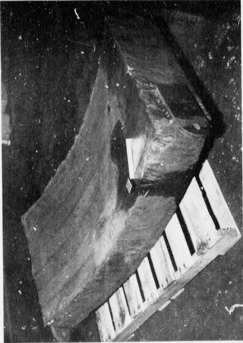
Fig. 7.23. Pilgrim Unit 2 pressure vessel piece (P-1) in which ultrasonic calibration reflectors are machined.
