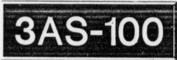
Exhibit 5. Ocone. Actual size of label for a component in the Unit 3 Auxiliary Steam system (Blue Background for Unit 3).
