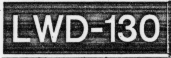
Exhibit 3. Ocone. Actual size of label for a component in the liquid waste drain system (Black Background for station common).
