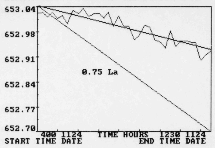
CALUERT CLIFFS - UNIT 2 ILRT MASS POINT LEAKAGE RATE AND UCL - %/DAY
