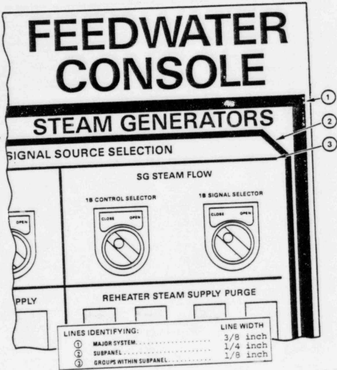
FIGURES 2-1. RECOMMENDED DEMARCATION LINE WIDTHS
