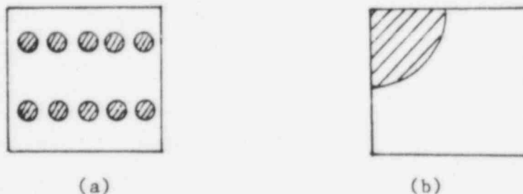
Fig. 5.7 Modeling (a) a Multiple or (b) a Fraction of a Structure as One Thermal Structure
