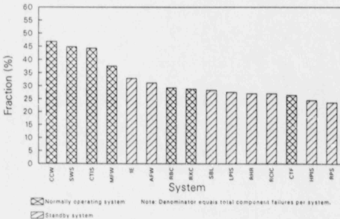
Figure 3. Fractions of the total failures within specified systems due to aging.
