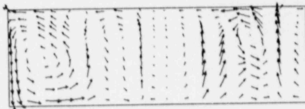
Figure 5.8 Velocity Contours at the First Vertical y-z Plane Near Ventilation Exit
