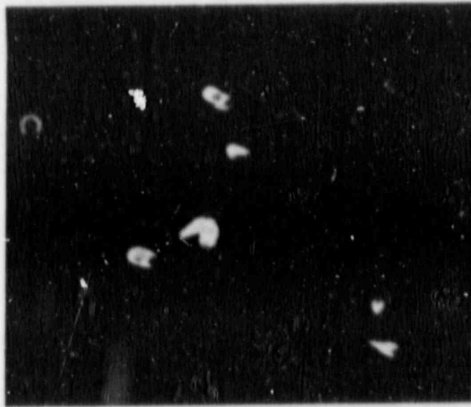
Figure 2. Autoradiograph of waste supernate after centrifugation to remove particles larger than 0.05 \mu\text{m} . The tracks are caused by alpha emitters unattached to visible particles. The emitters are probably plutonium and are probably chelated, thus they do not sorb and remain in solution---designated soluble fraction.
