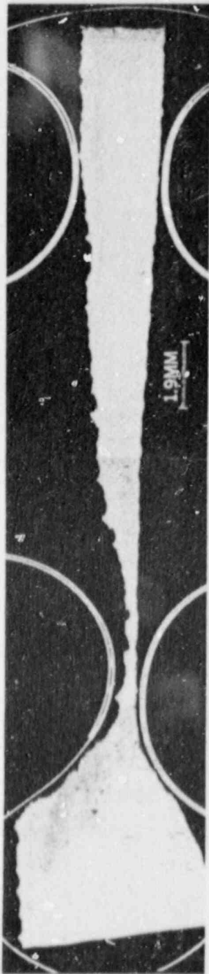
Figure 24. Photomicrograph of a cross section of the "worn" area near the weld on specimen 1A-4. The thinnest area measured approximately .015 inch (0.38 mm).
