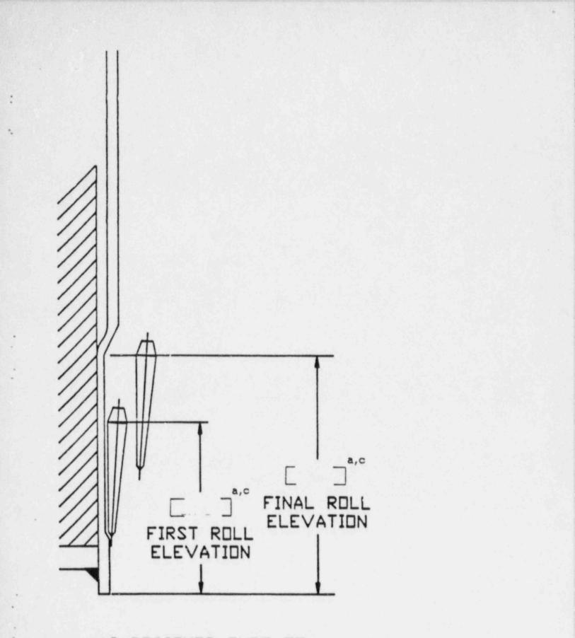
AS DESIGNED TUBE TO TUBESHEET ROLL GEOMETRY
