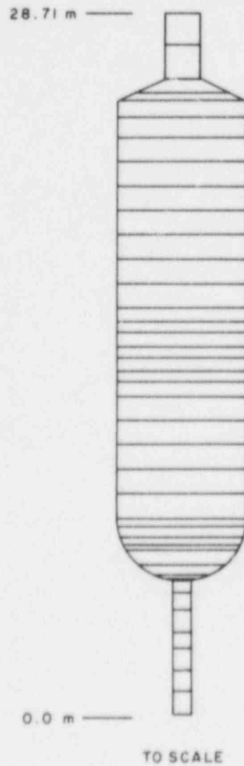
Figure 2.3.1 Nodalization for Marviken Vessel and Discharge Pipe.
