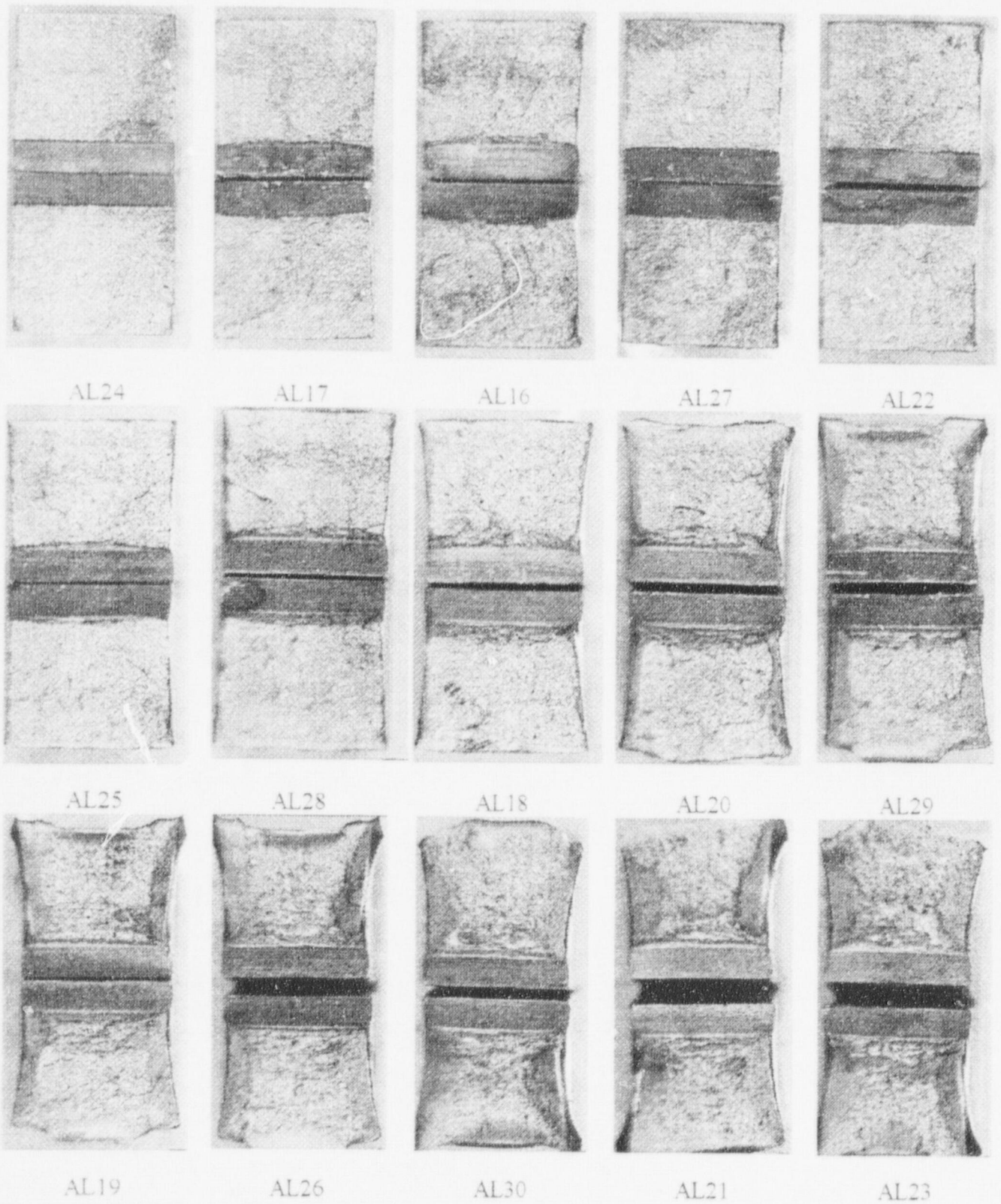
Figure 5-13 Charpy Impact Specimen Fracture Surfaces for Vogtle Unit 1 Reactor Vessel Intermediate Shell Plate B8805-3 (Longitudinal Orientation)
