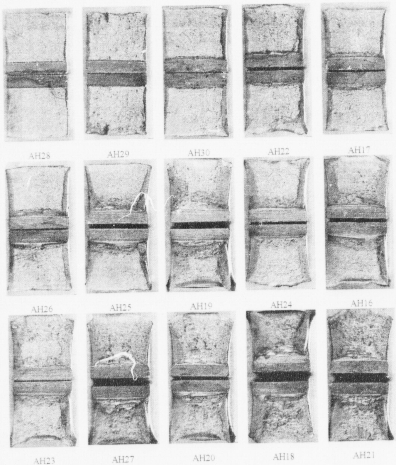
Figure 5-16 Charpy Impact Specimen Fracture Surfaces for Vogtle Unit 1 Reactor Vessel Heat-Affected-Zone Metal
