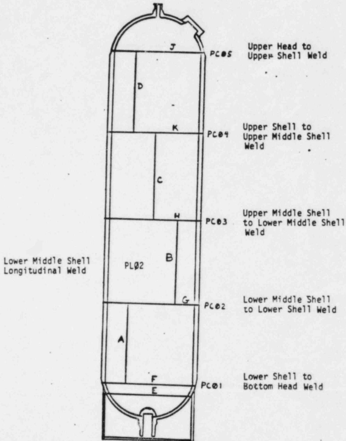
Figure 5-1 Schematic of Byron Unit 2 D-84 Series Pressurizer
