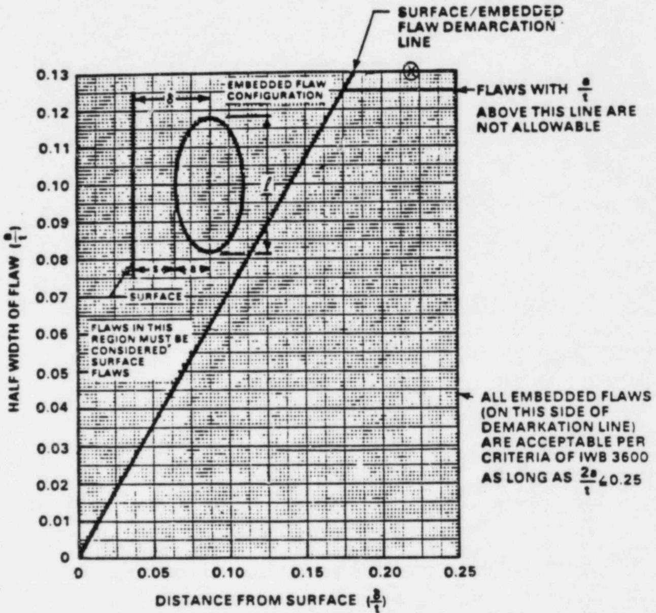
Figure 4-2 Example of Embedded Flaw Evaluation Chart
