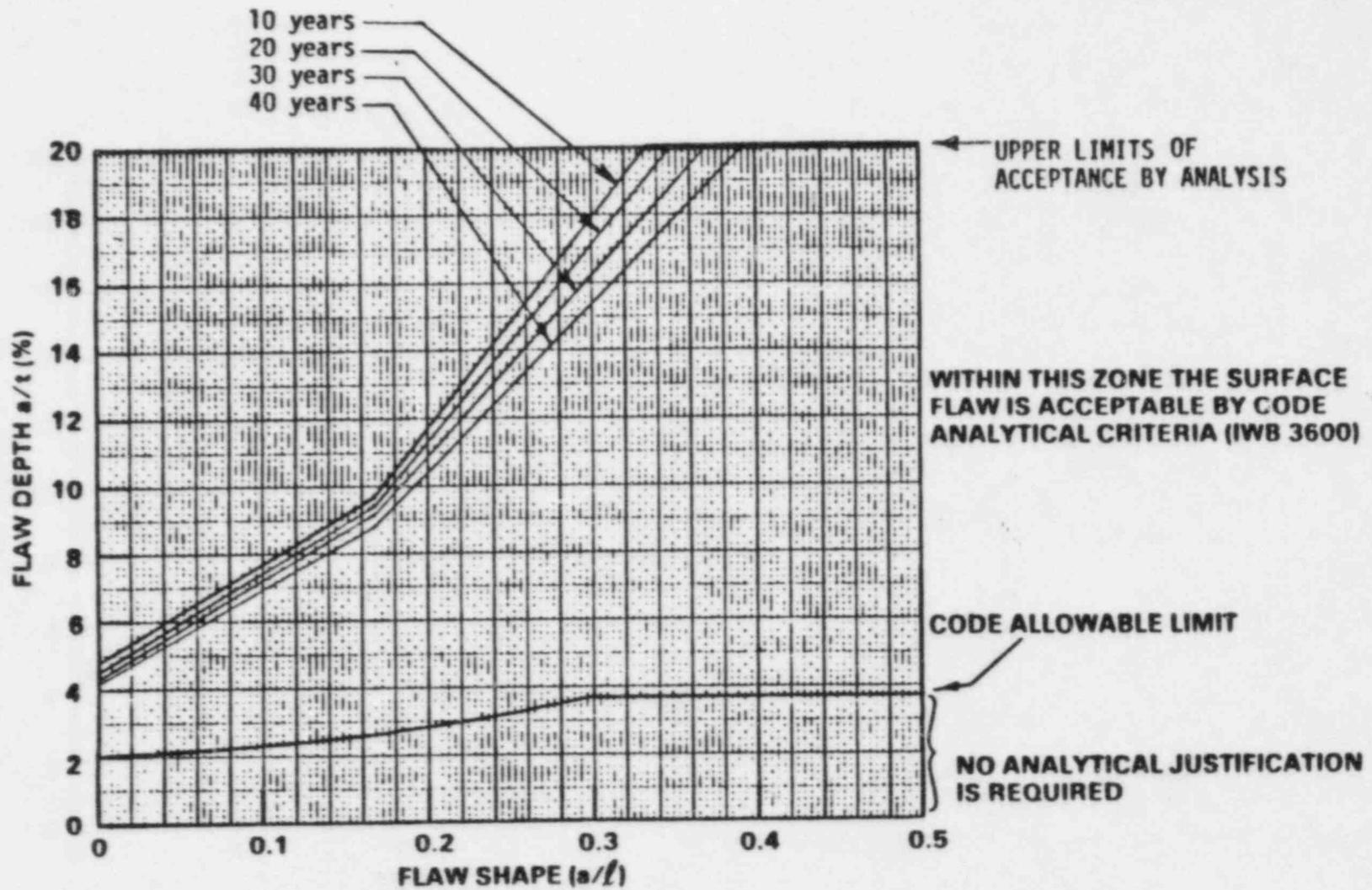
FIGURE 4-1 Flaw Evaluation Chart for Circumferential Surface Flaw in the Tube Sheet to Stub Barrel Weld Region
