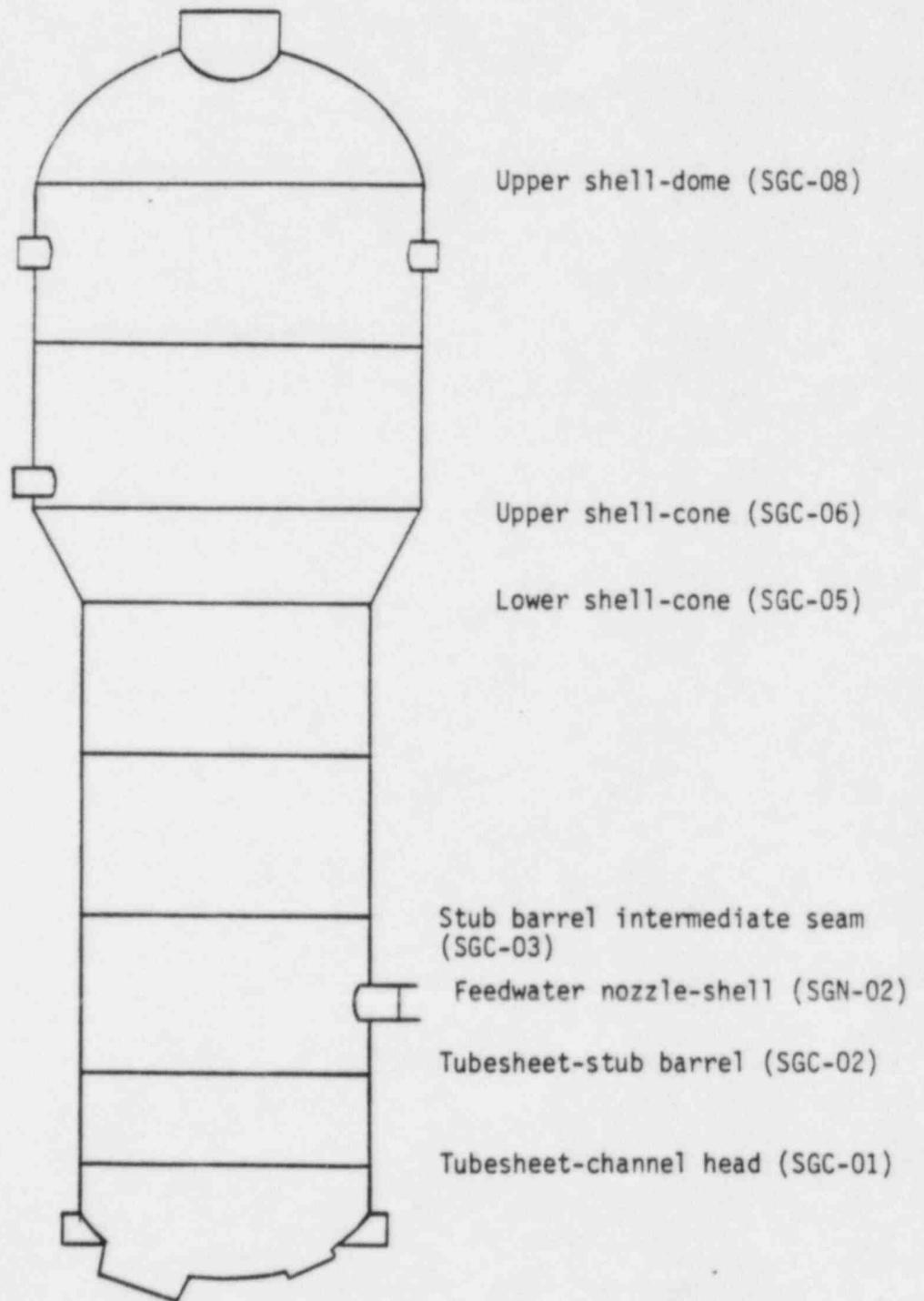
Figure 1-1 Schematic of Byron Unit 2 Model D-5 Steam Generator
