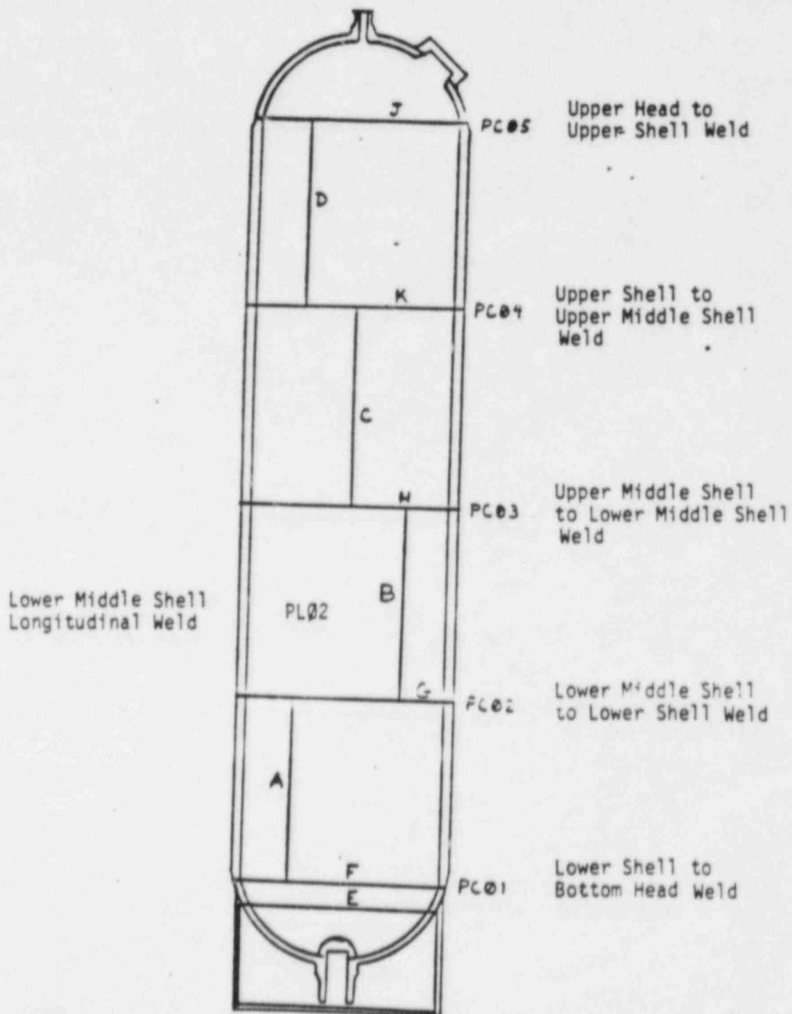
Figure 1-1 Schematic of Byron Unit 2 D-84 Series Pressurizer
