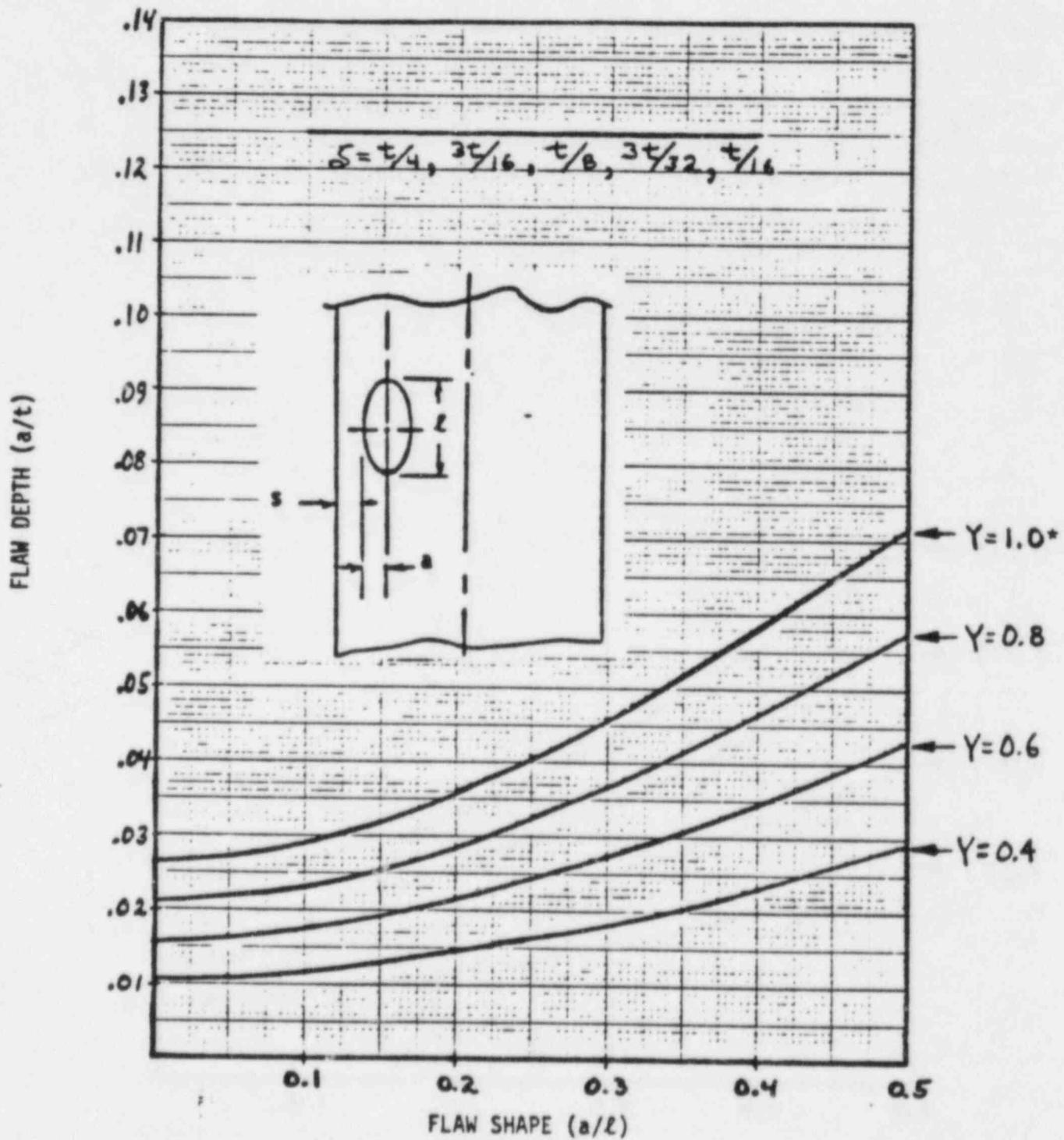
FIGURE 4-3 Acceptance Standards for Embedded Flaws, from Table IWB-3511-1
