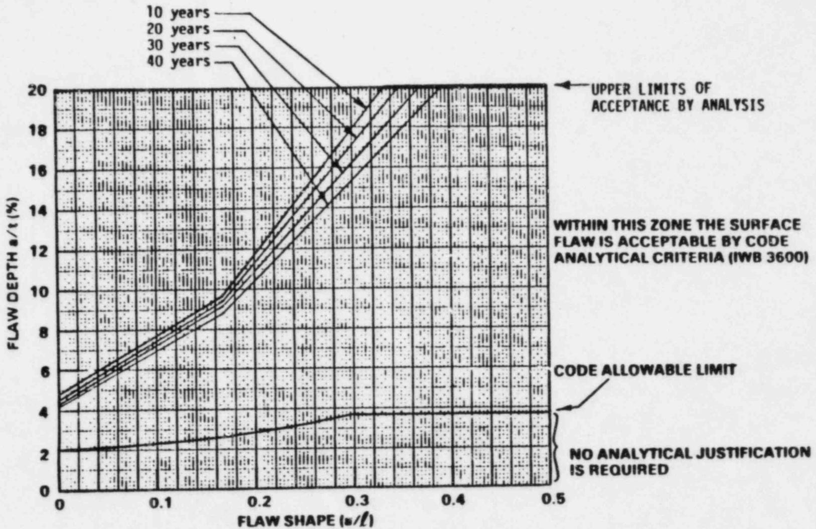
FIGURE 4-1 Example of Surface Flaw Evaluation Chart
