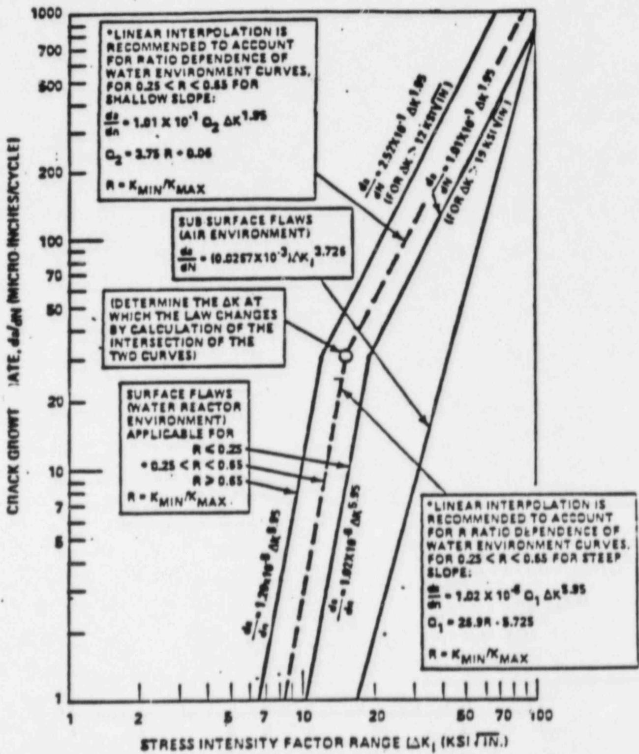
FIG. 3-1 REFERENCE FATIGUE CRACK GROWTH CURVES FOR CARBON AND LOW ALLOY FERRITIC STEELS
