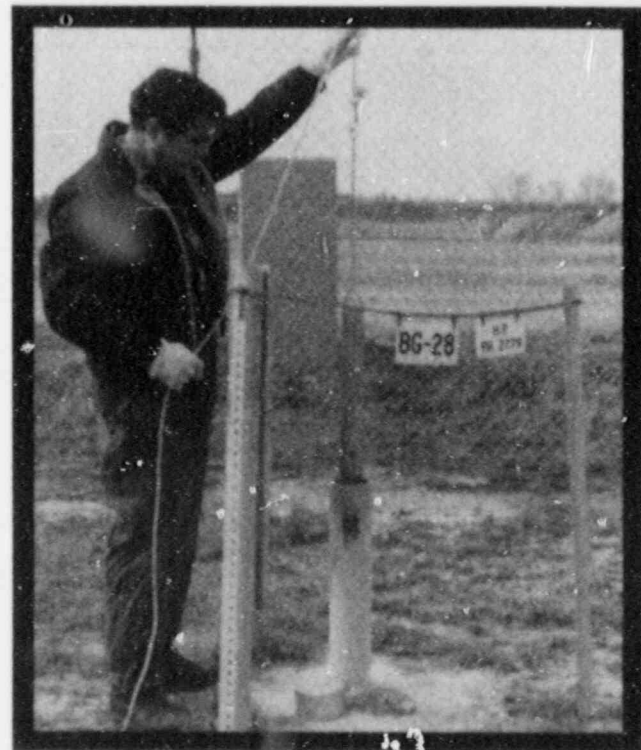
Wells monitor Burial Ground perimeter
