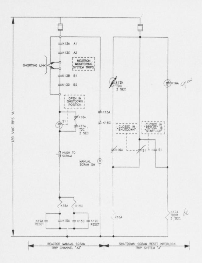
Figure 03-21 - Shutdown Scram Reset Interlock
