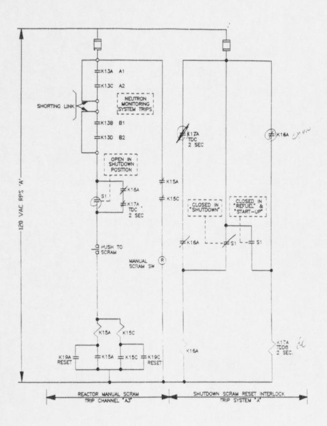
Figure 03-21 - Shutdown Scram Reset Interlock
