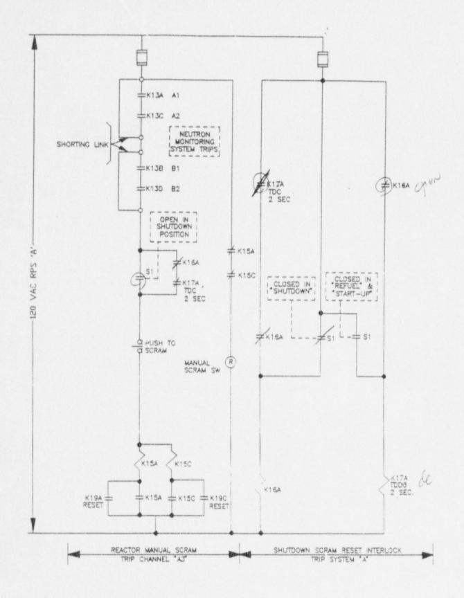
Figure 03-21 - Shutdown Scram Reset Interlock
