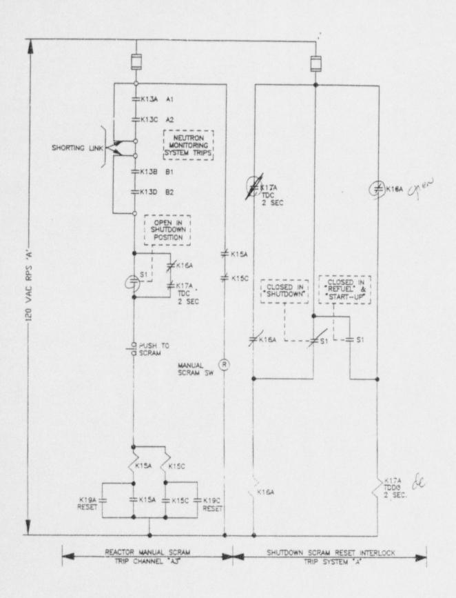
Figure 03-21 - Shutdown Scram Reset Interlock
