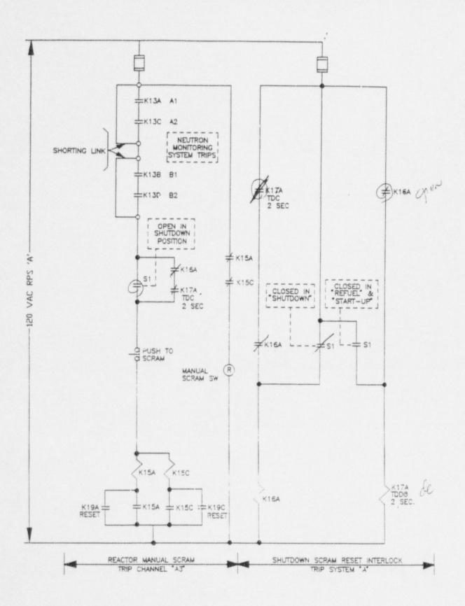
Figure 03-21 - Shutdown Scram Reset Interlock
