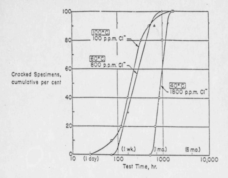
Figure 1. Effect of temperature on the time to cracking of Type 304 stainless steel exposed to water with chloride adjusted to provide the same rate of chloride concentration at three temperatures.
