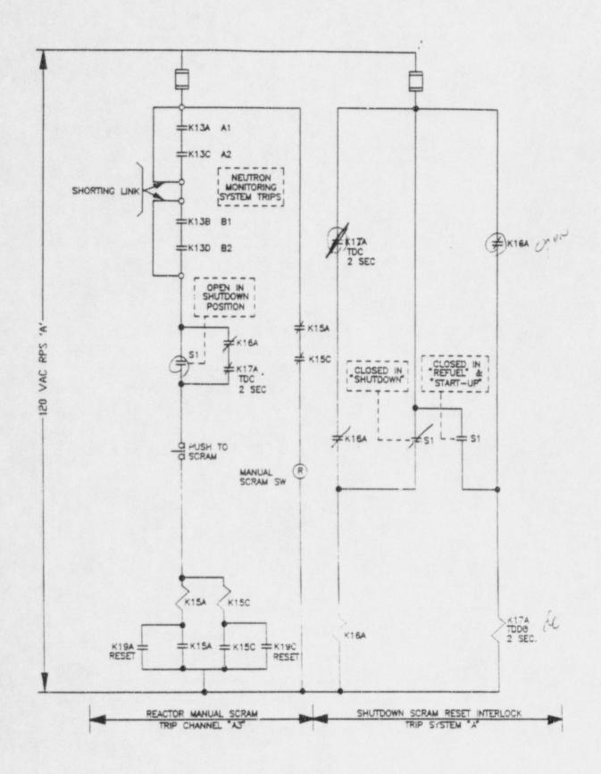
Figure 03-21 - Shutdown Scram Reset Interlock
