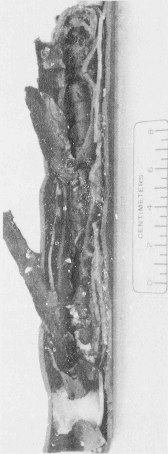
Fig. 10. Posttest view of the simulated fuel specimen used in test HS-4.
