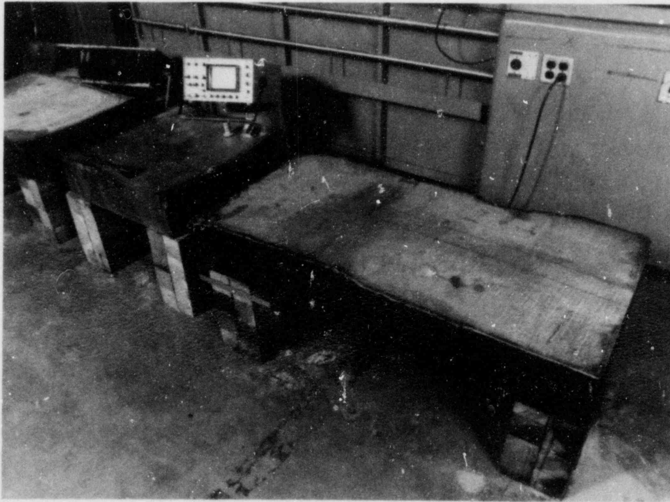
Fig. 7.1. Section of pressure vessel from Hope Creek Unit 2 reactor with ultrasonic equipment.
