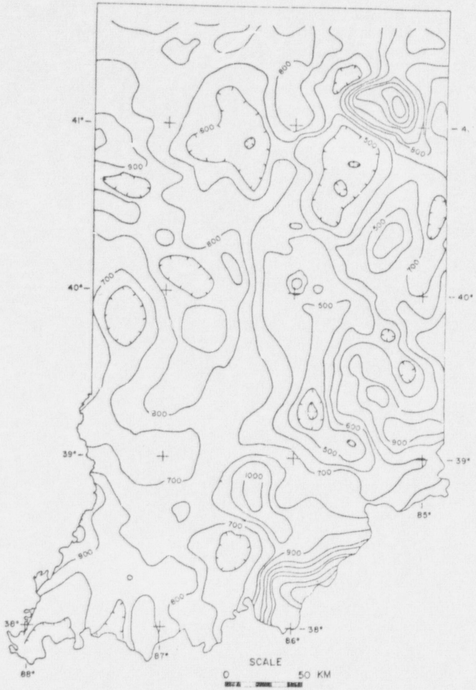
INDIANA AEROMAGNETIC ANOMALY MAP REDUCED TO THE POLE, UPWARD CONTINUED TO 5 KM CONTOUR INTERVAL = 100 GAMMAS
