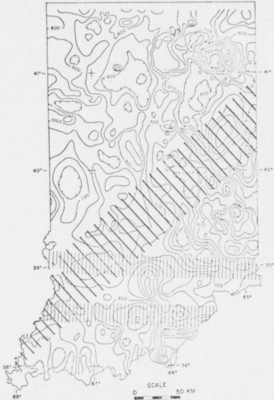
INDIAN AEROMAGNETIC ANOMALY MAP REDUCED TO THE POLE, UPWARD CONTINUED TO 2 KM CONTOUR INTERVAL 100 GAMMAS
