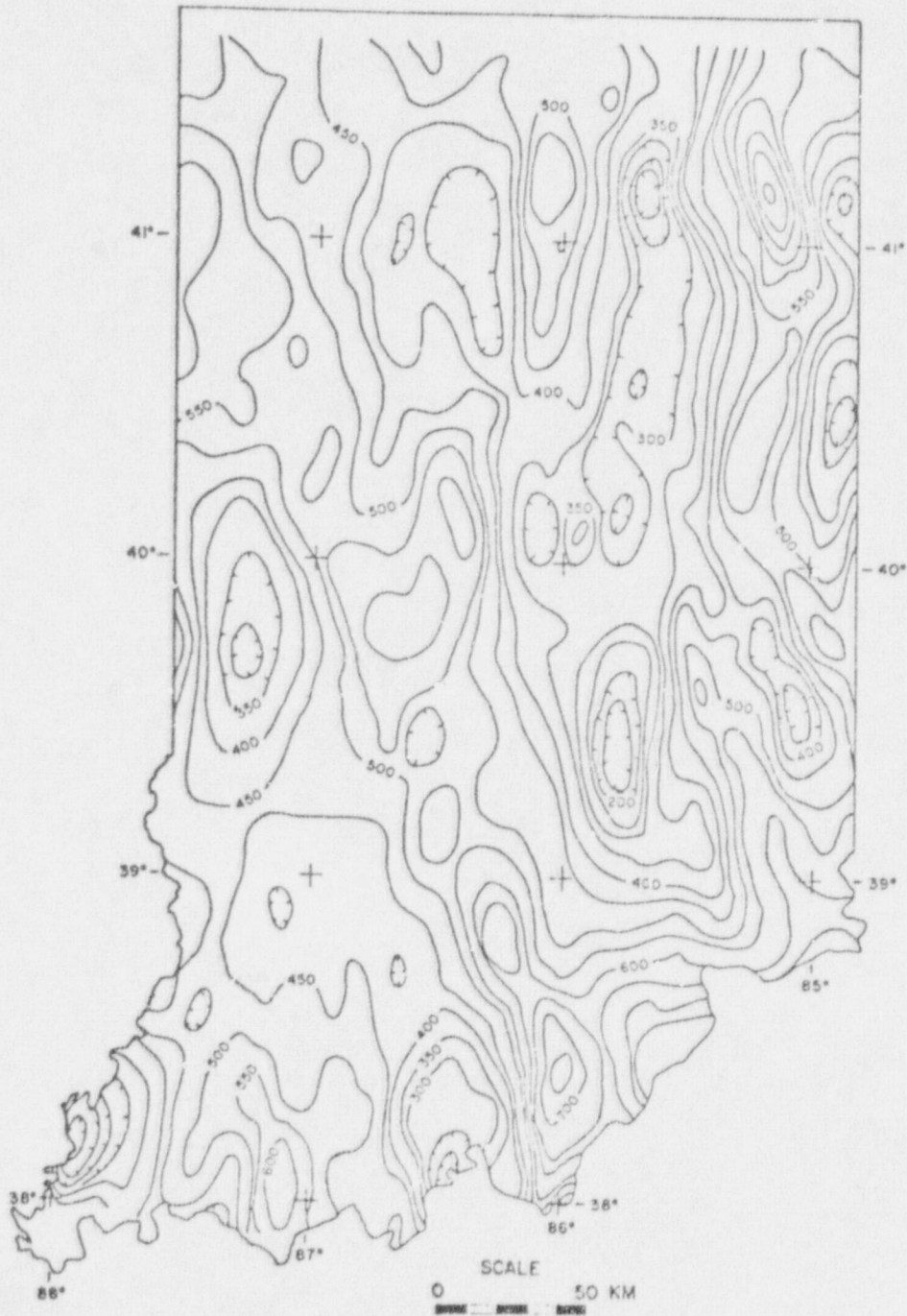
INDIANA AEROMAGNETIC ANOMALY MAP UPWARD CONTINUED TO 5 KM, N-S STRIKE PASS CONTOUR INTERVAL = 50 GAMMAS
