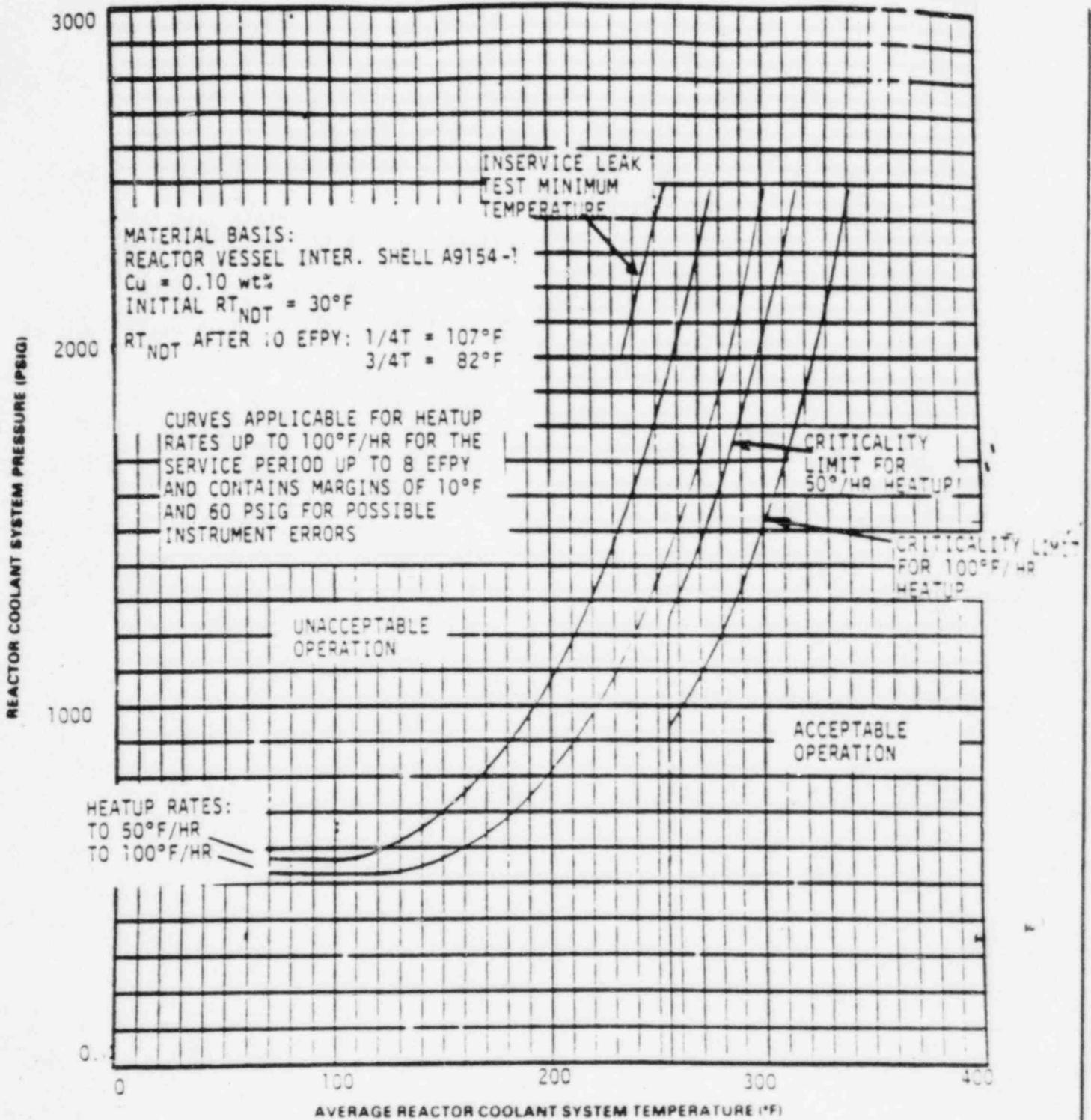
Figure 3-4-2 Reactor Coolant System Pressure - Temperature Limits Versus 100°F/Hour and 50°F/Hour Heatup Rate - Criticality Limit and Inservice Leak Test Limit
