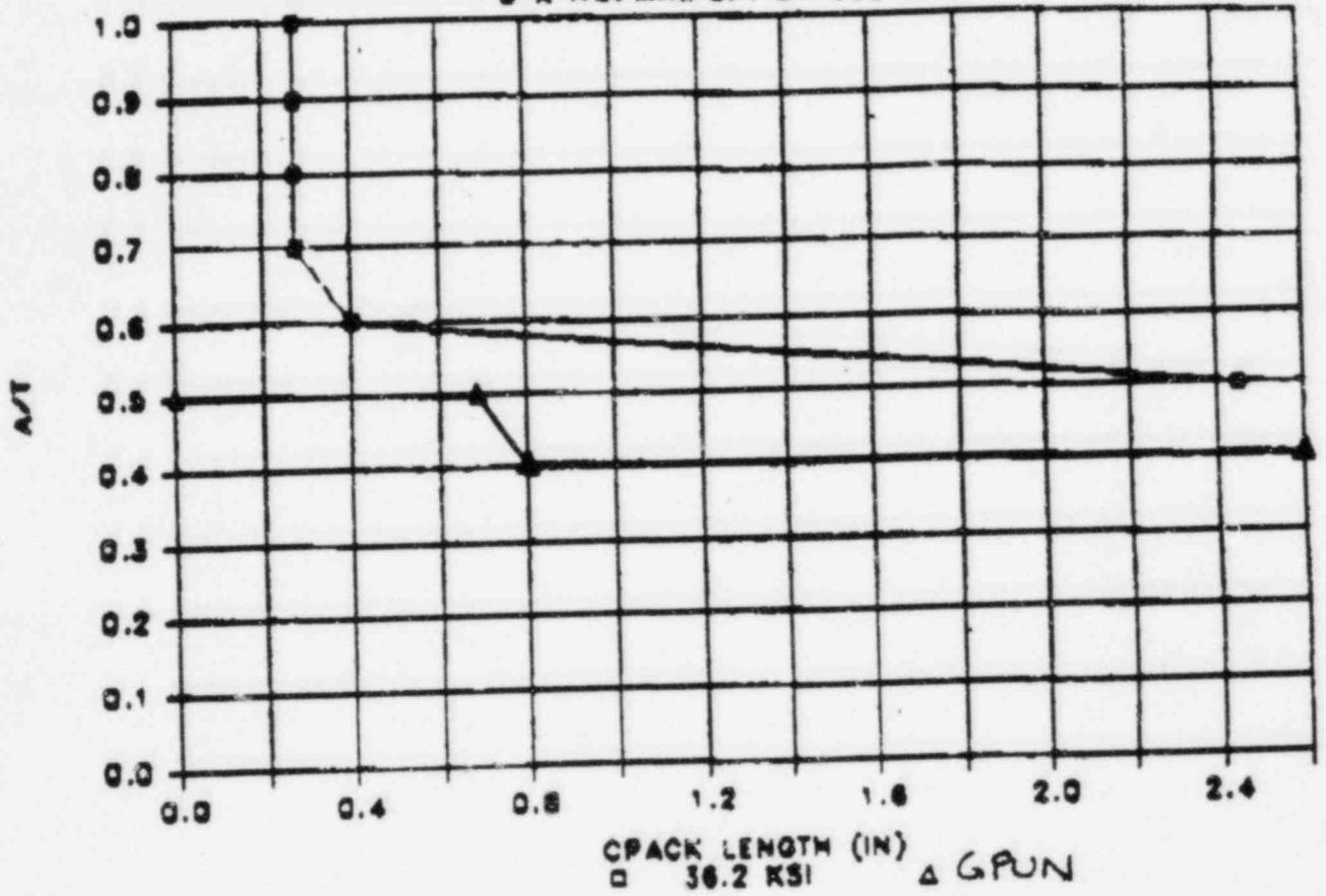
Net Section Collapse Criterion Results for Axial Cracks
