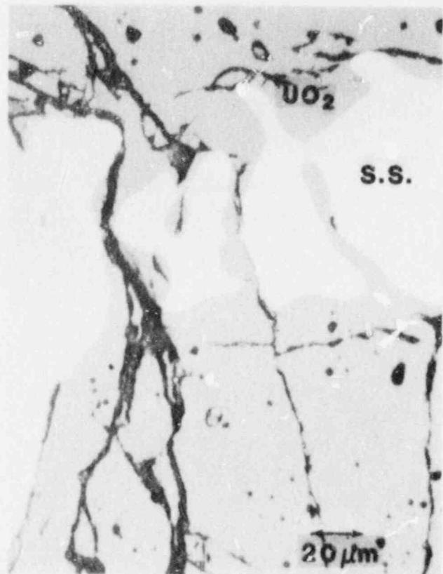
b. Layer structure steel and UO_2 fingers. Same area at higher magnification.
