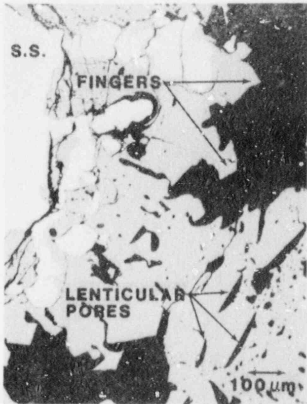
a. Vapor transported UO_2 and steel contiguous with large steel globule. Location (20,42).
