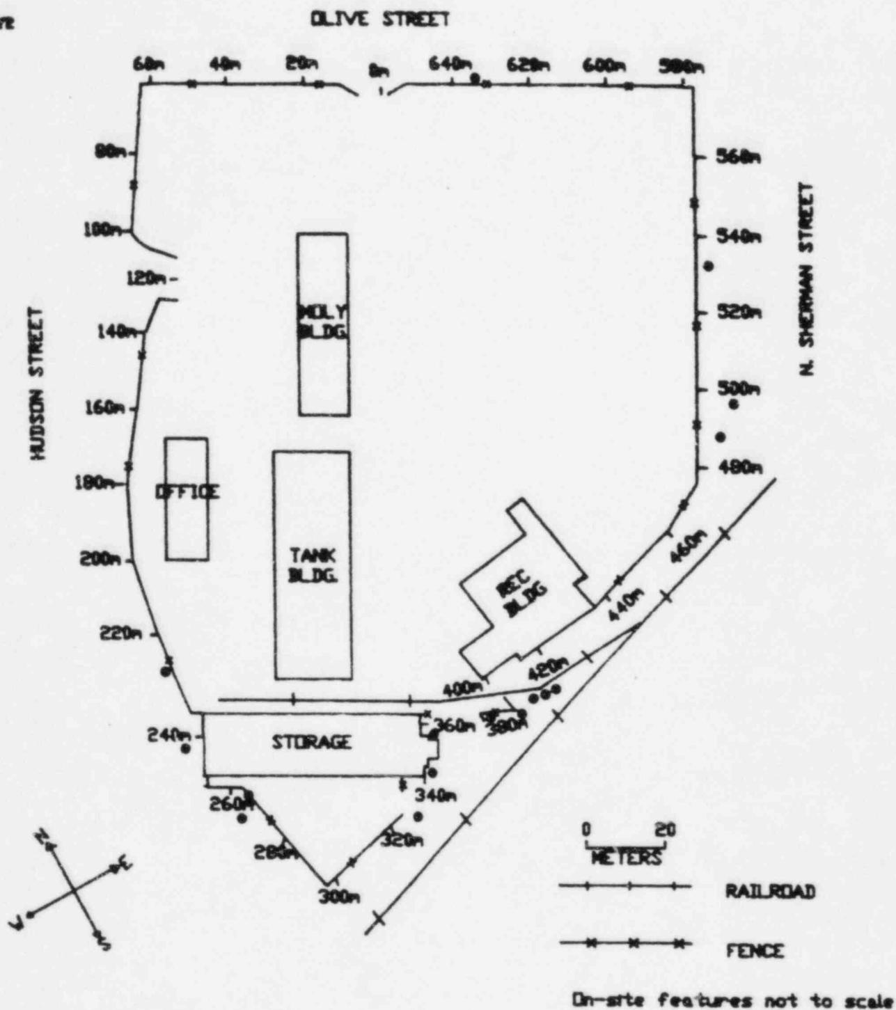
FIGURE 13: Locations (●) of Areas of Elevated Direct Radiation Identified by the Walkover Surface Scan.
