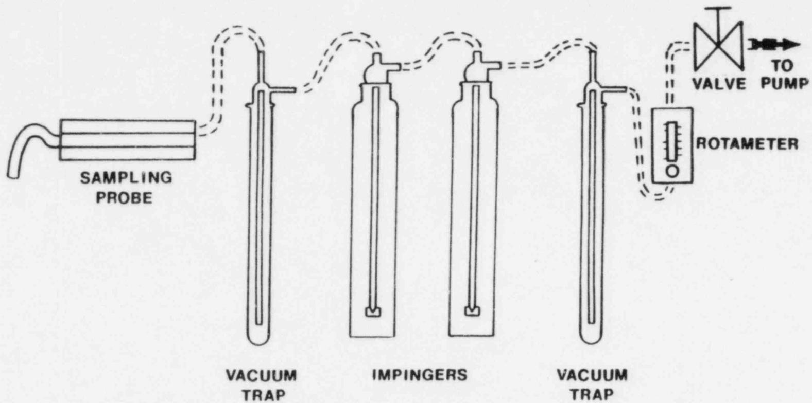
FIGURE 11: Diagram of the Sampling System for the Tank and REC Building Scrubbers.
