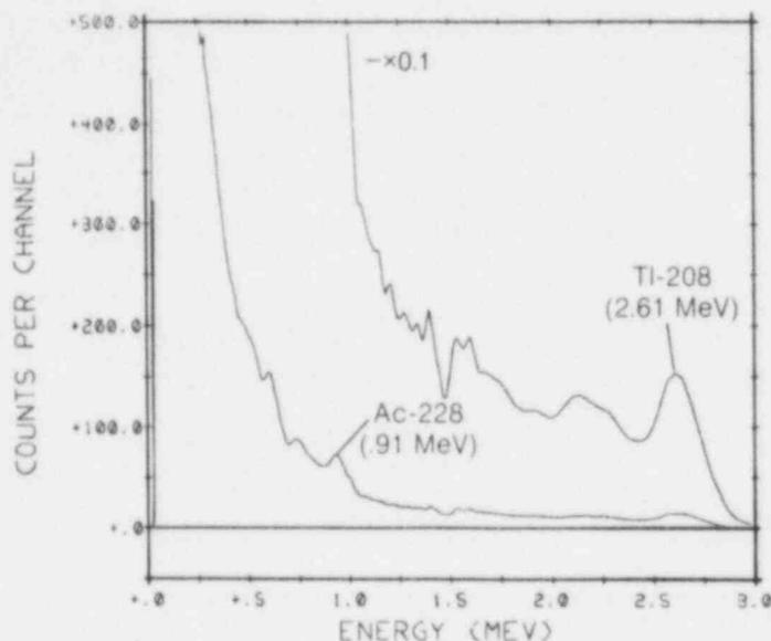
Figure 8. BACKGROUND-SUBTRACTED GAMMA RAY SPECTRUM OBTAINED OVER THE MOLYCORP, INC. FACILITY
