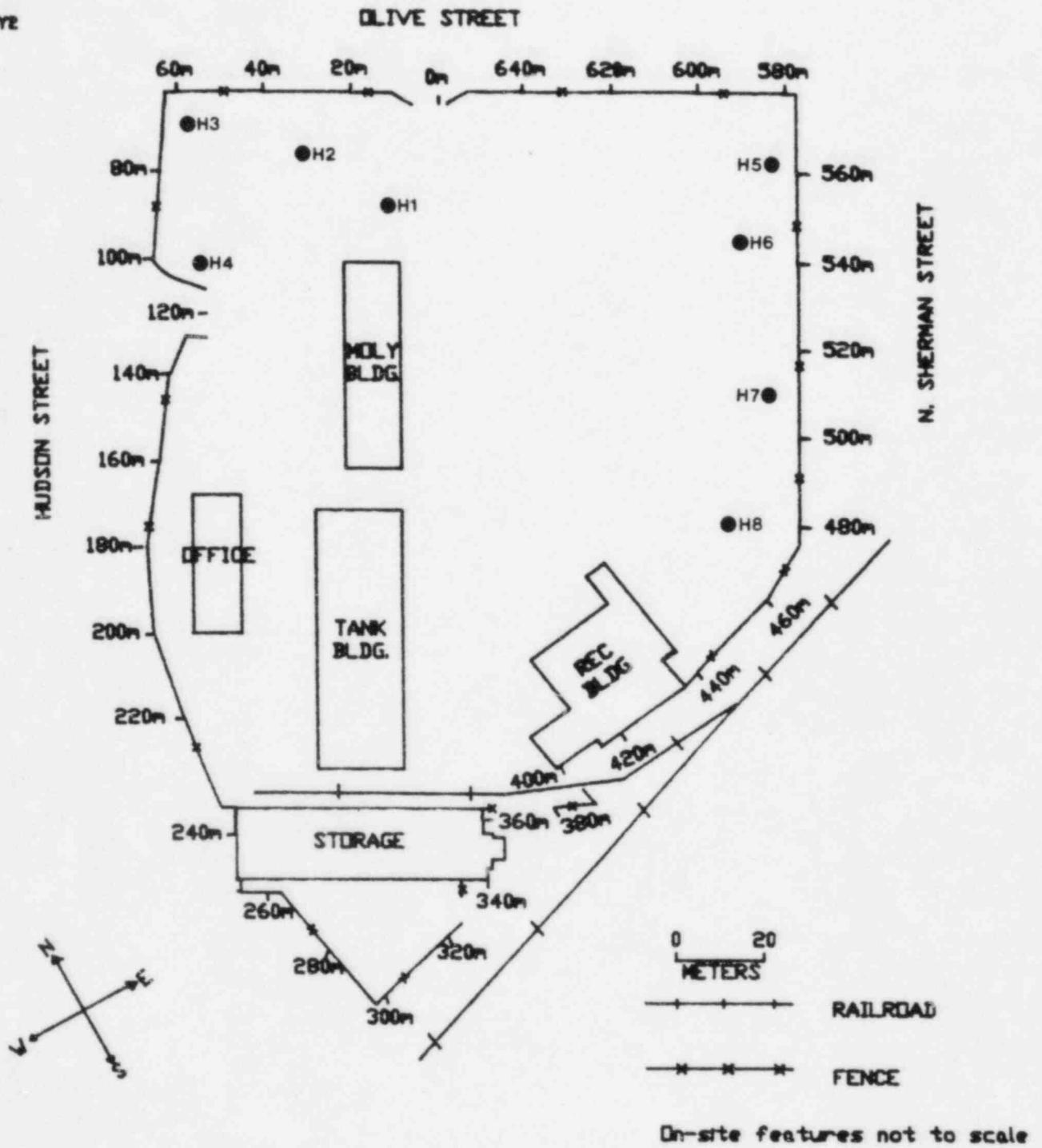
FIGURE 4 Locations of Boreholes for Subsurface Investigations.
