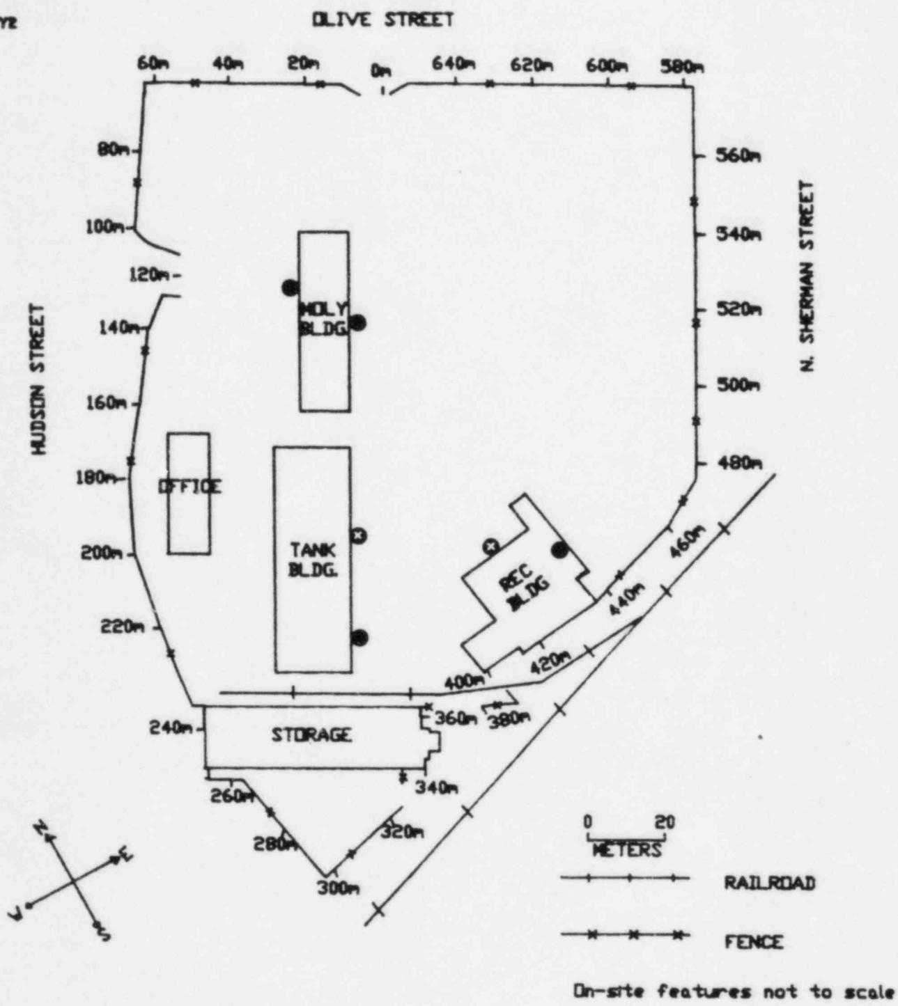
FIGURE 9: Layout of the Molybdenum Corporation of America Plant Showing Dust Collector and Scrubber Locations. (Locations marked with an "X" indicate ORAU sampling points.)
