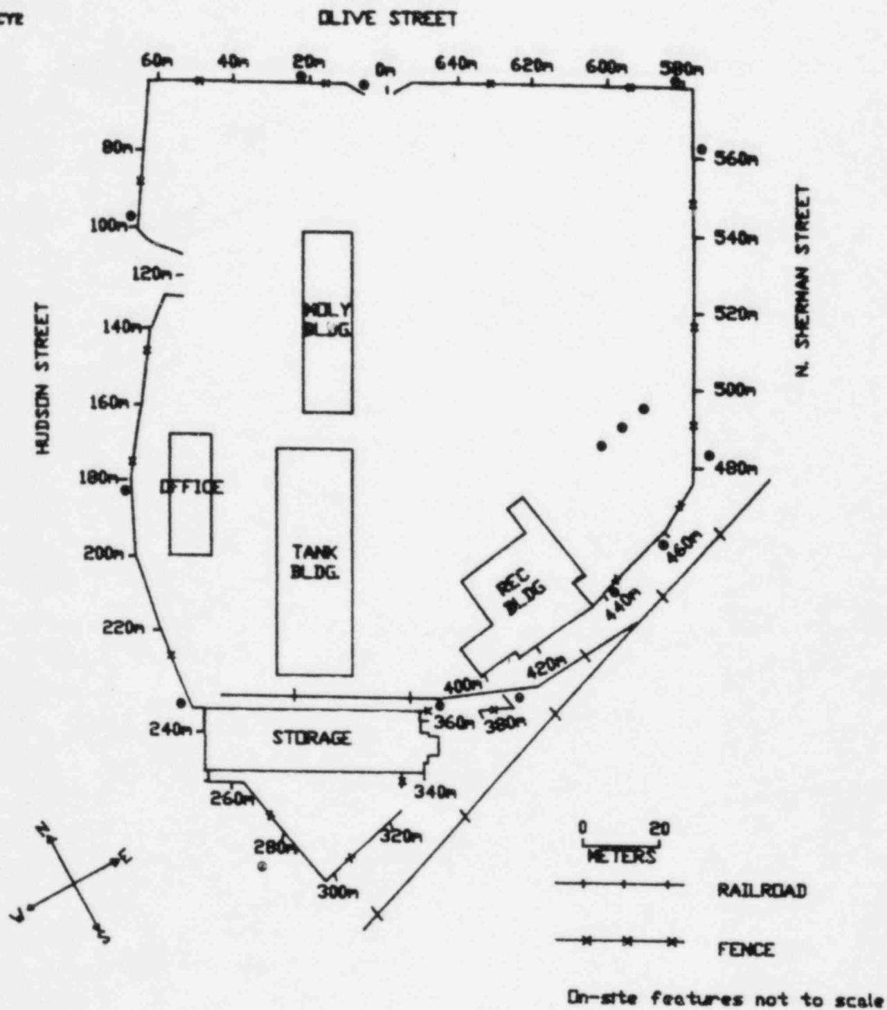
FIGURE 3: Locations (●) of Measurements for Calibration of the NaI Scintillation Detectors.
