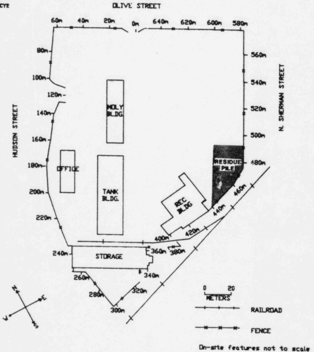
FIGURE 2: Map of the Layout of the Molybdenum Corporation of America Plant Indicating Prominent Surface Features and the Reference System Used for Survey Measurements.
